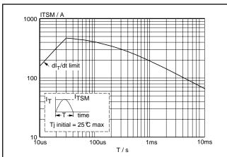
Fig.2. Maximum permissible non-repetitive peak on-state current  $I_{TSM}$ , versus pulse width  $t_p$ , for sinusoidal currents,  $t_p \le 10$ ms.
