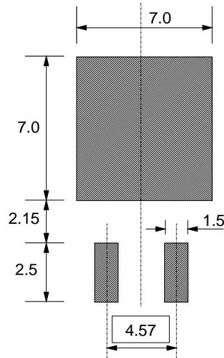
Fig.14. SOT428 : minimum pad sizes for surface mounting.
