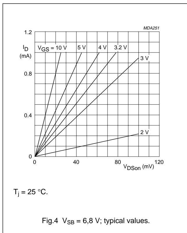
Fig.4  $V_{SB} = 6.8$  V; typical values.
