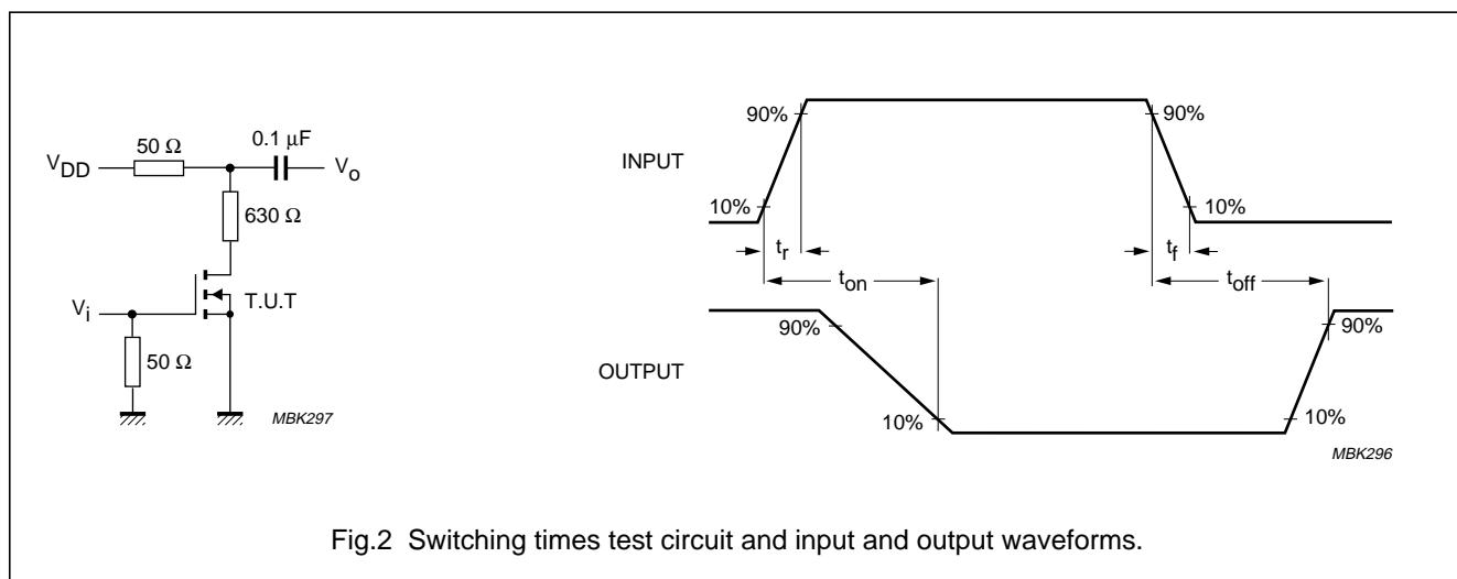
Fig.2 Switching times test circuit and input and output waveforms.
