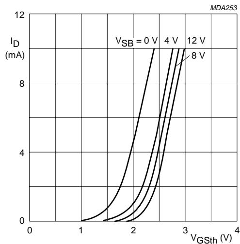
$T_j = 25^\circ\text{C}$ .Fig.6  $V_{DS} = V_{GS} = V_{GS(\text{th})}$ .
