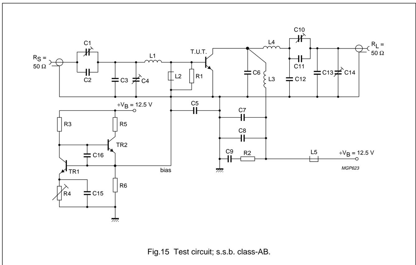
Fig.15 Test circuit; s.s.b. class-AB.
