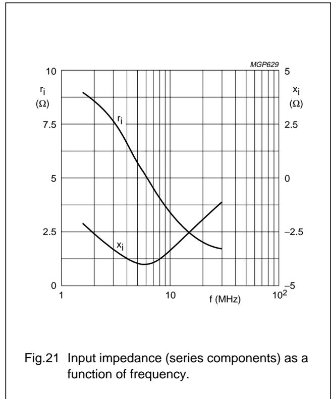
Fig. 20 and 21 are typical curves and hold for an unneutralized amplifier in s.s.b. class-AB operation.
