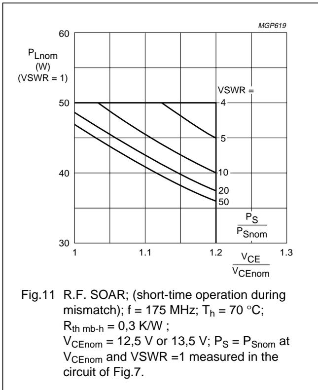
The transistor has been developed for use with unstabilized supply voltages. As the output power and drive power increase with the supply voltage, the nominal output power must be derated in accordance with the graph for safe operation at supply voltages other than the nominal. The graph shows the permissible output power under nominal conditions ( $VSWR = 1$ ), as a function of the expected supply over-voltage ratio with  $VSWR$  as parameter.
