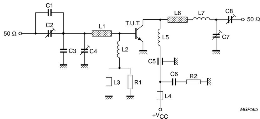
Fig.7 Class-B test circuit at  $f = 470\text{ MHz}$ .
