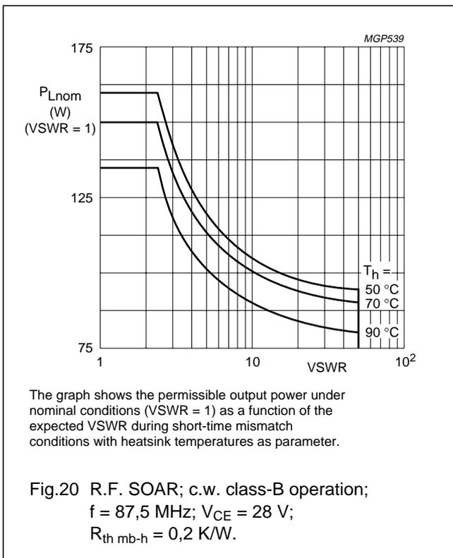
The graph shows the permissible output power under nominal conditions (VSWR = 1) as a function of the expected VSWR during short-time mismatch conditions with heatsink temperatures as parameter.
