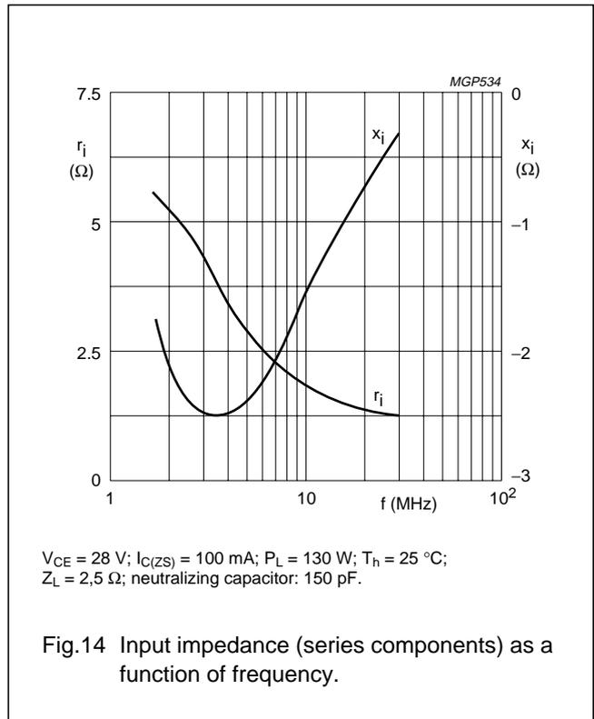
13 and 14 are typical curves and hold for a push-pull amplifier with cross-neutralization in s.s.b class-AB operation.
