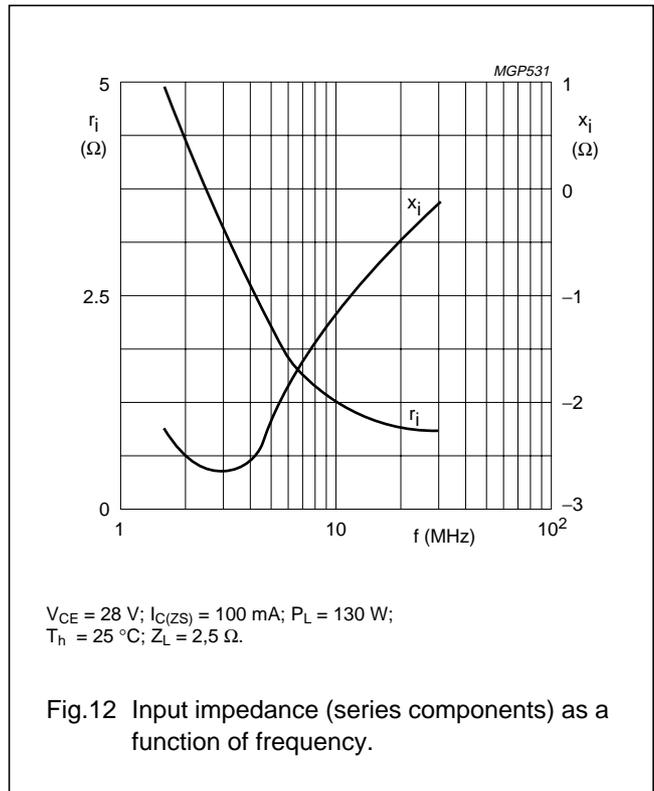
Figs 11 and 12 are typical curves and hold for an unneutralized amplifier in s.s.b. class-AB operation.
