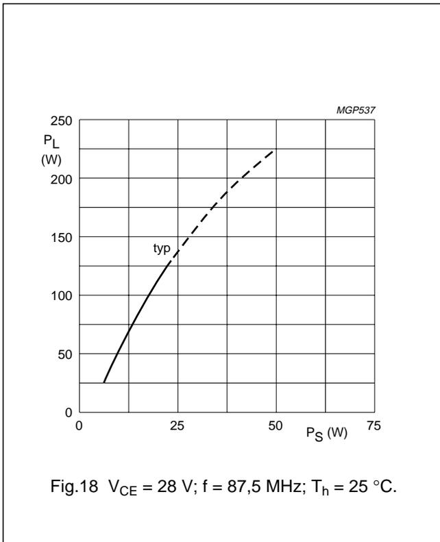
Fig.18  $V_{CE} = 28$  V;  $f = 87,5$  MHz;  $T_h = 25$  °C.
