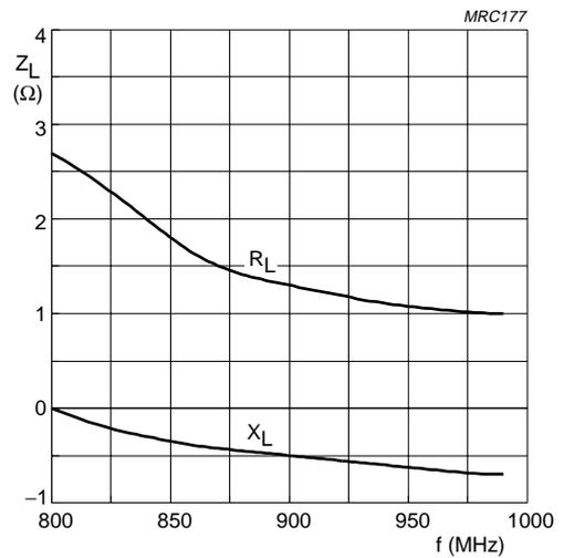
Fig.11 Load impedance; series components;
