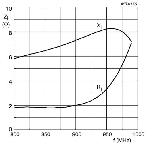
Fig.10 Input impedance; series components;
