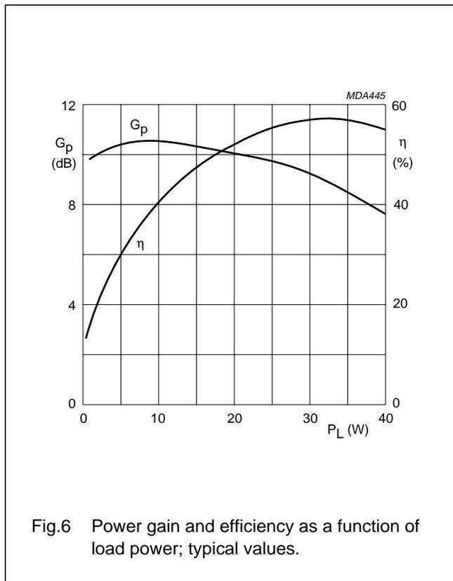
Fig.6 Power gain and efficiency as a function of load power; typical values.
