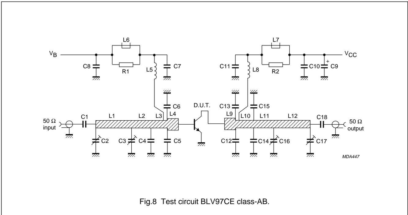
Fig.8 Test circuit BLV97CE class-AB.
