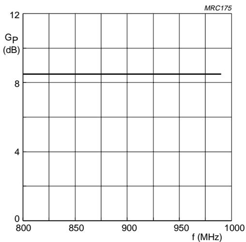
Fig.12 Power gain; class-AB operation;
