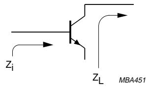
Fig.12 Definition of transistor impedance.
