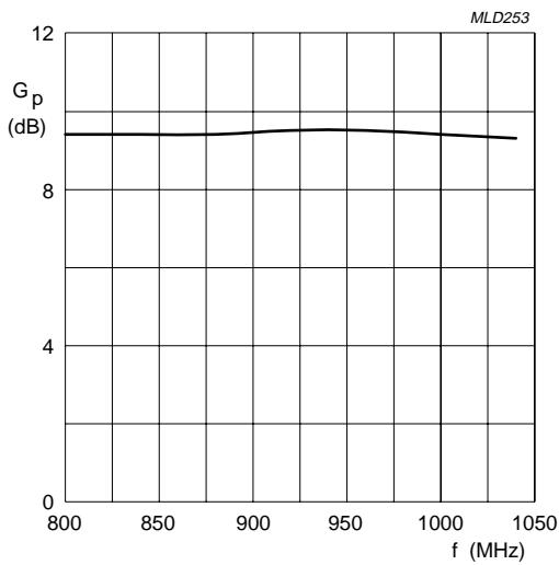
$V_{CE} = 26$  V;  $I_{CQ} = 200$  mA;  $P_L = 75$  W;
