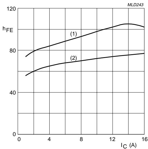
Measured under pulsed conditions;  $t_p \leq 500 \mu\text{s}$ ;  $\delta \leq 0.01$ .(1)  $V_{\text{CE}} = 26 \text{ V}$ .(2)  $V_{\text{CE}} = 10 \text{ V}$ .
