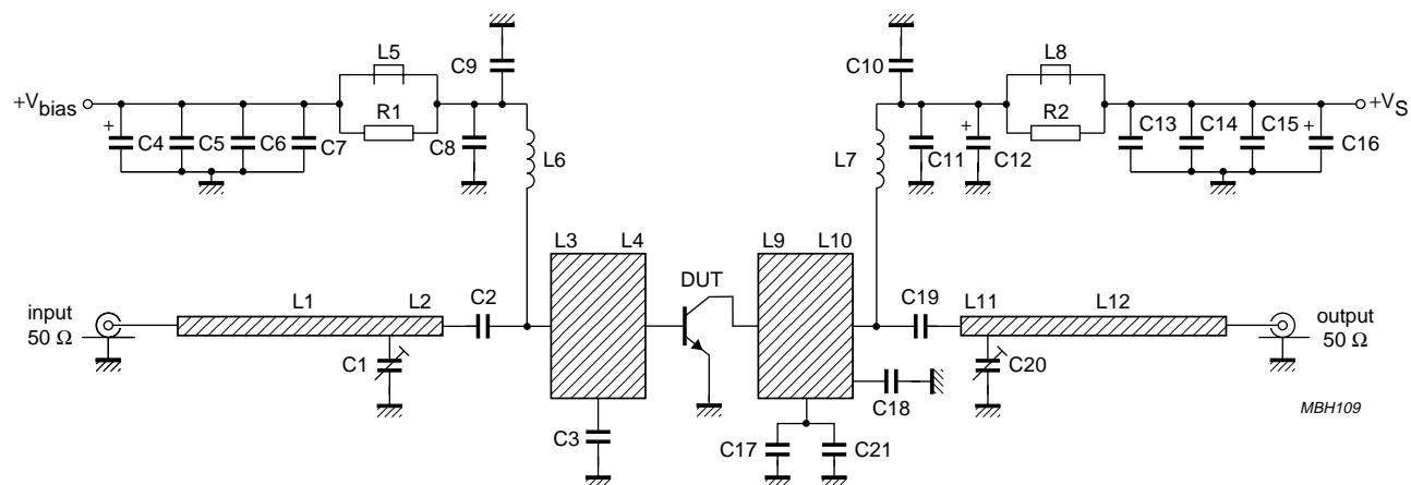
Fig.7 Class-AB test circuit at  $f = 960$  MHz.
