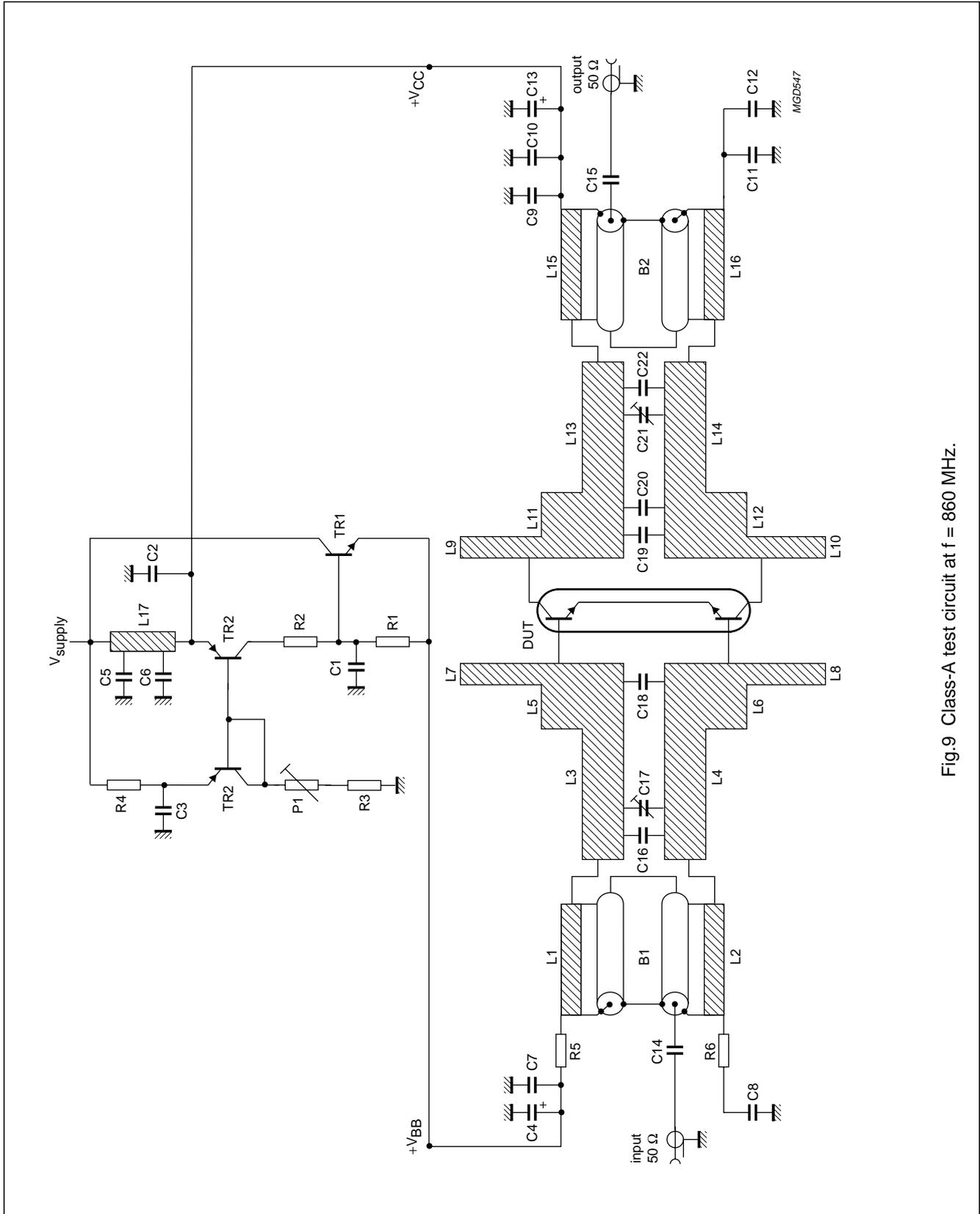
Fig.9 Class-A test circuit at f = 860 MHz.
