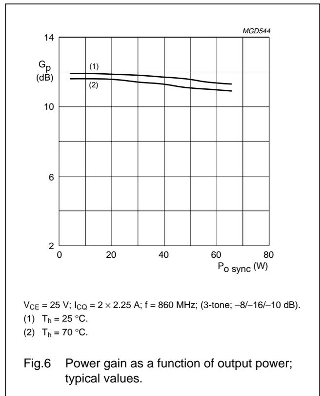
UHF linear push-pull power transistor
