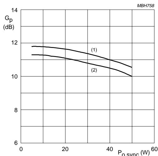
$V_{CE} = 25$  V;  $I_{CQ} = 2 \times 1.1$  A;  $f = 860$  MHz; (3-tone;  $-8/-16/-10$  dB).
