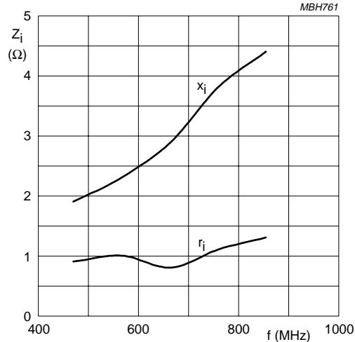
$V_{CE} = 25$  V;  $I_{CQ} = 2 \times 1.1$  A;  $P_{o\ sync} = 10$  W (total device);  $T_h = 25$  °C.
