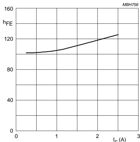
$V_{\text{CE}} = 25 \text{ V}; t_p = 500 \mu\text{s}; \delta = <1 \text{ \%}$ .
