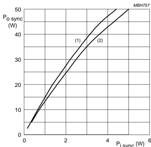
$V_{CE} = 25$  V;  $I_{CQ} = 2 \times 1.1$  A;  $f = 860$  MHz; (3-tone;  $-8/-16/-10$  dB).
