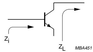
Fig.14 Definition of transistor impedance.
