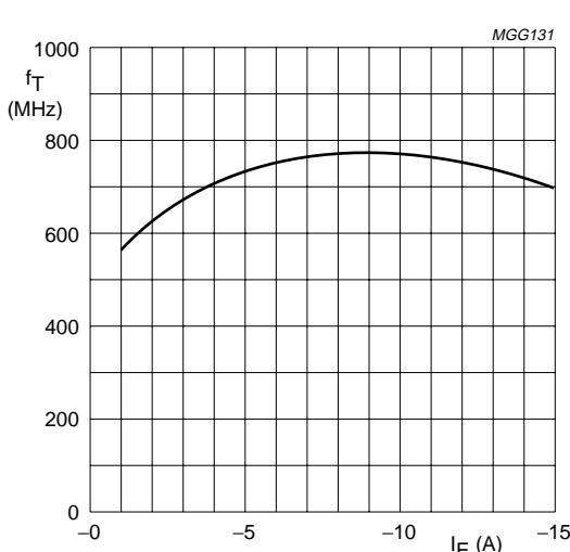
$V_{CB} = 25$  V;  $f = 100$  MHz;  $T_j = 25$  °C.
