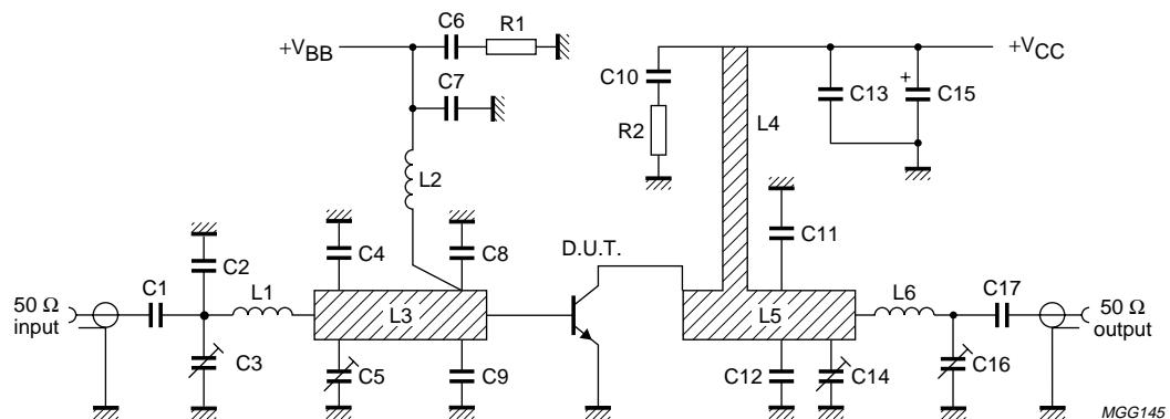
Fig.16 Class-AB test circuit at f<sub>vision</sub> = 224.25 MHz.
