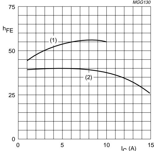
$T_j = 25$  °C.(1)  $V_{CE} = 25$  V.(2)  $V_{CE} = 5$  V.
