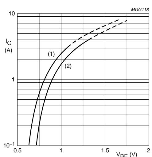
$V_{CE} = 25$  V.(1)  $T_h = 70$  °C.(2)  $T_h = 25$  °C.
