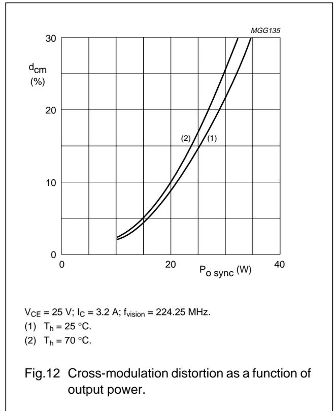
Three-tone test method (vision carrier  $-8\text{ dB}$ , sound carrier  $-7\text{ dB}$ , sideband signal  $-16\text{ dB}$ ), zero dB corresponds to peak sync level (see Fig.11). Intermodulation distortion of input signal  $\leq -70\text{ dB}$ .
