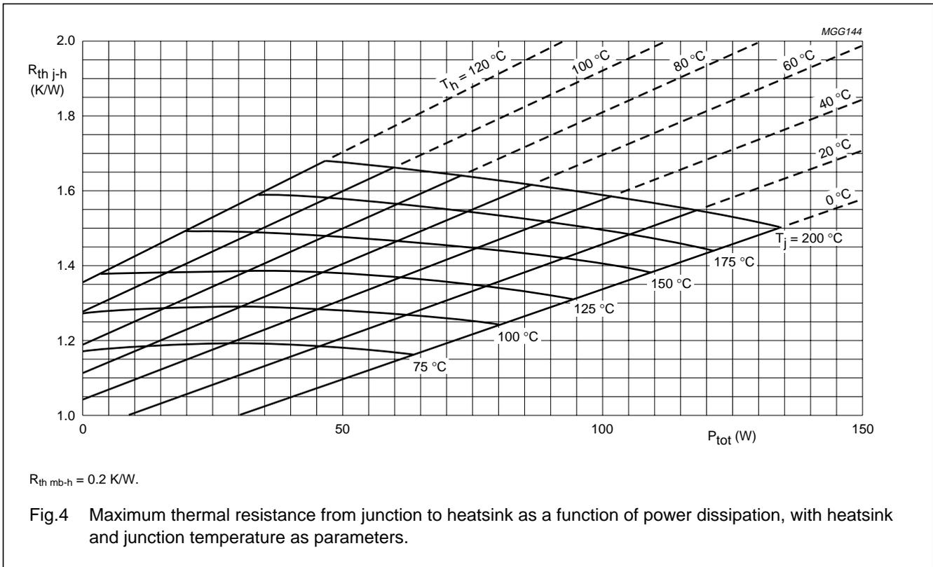
Fig.4 Maximum thermal resistance from junction to heatsink as a function of power dissipation, with heatsink and junction temperature as parameters.
