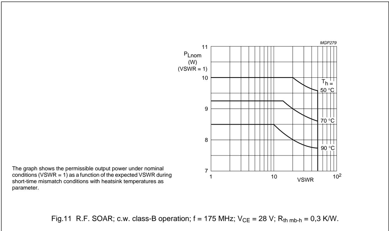
The graph shows the permissible output power under nominal conditions ( $VSWR = 1$ ) as a function of the expected VSWR during short-time mismatch conditions with heatsink temperatures as parameter.
