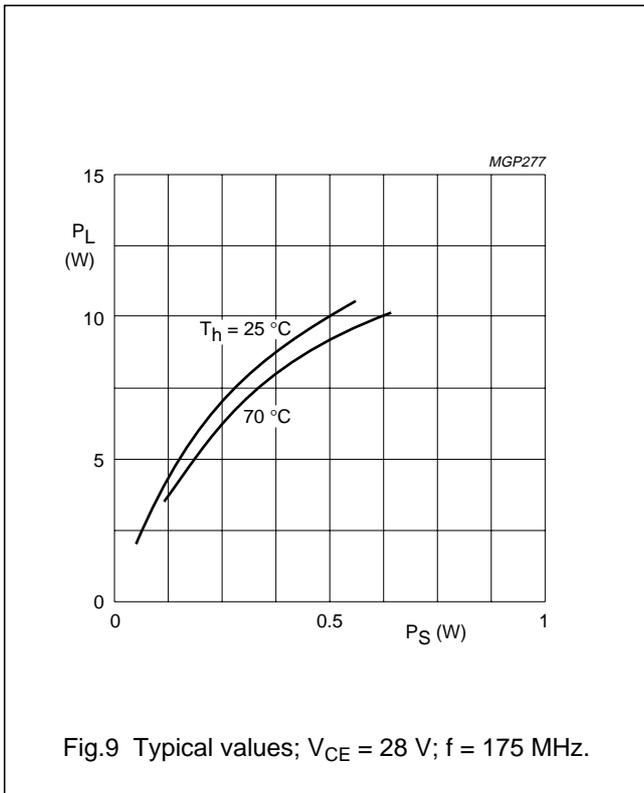
Fig.9 Typical values;  $V_{CE} = 28\text{ V}$ ;  $f = 175\text{ MHz}$ .
