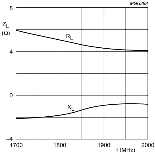
$V_{CE} = 26$  V;  $I_{CQ} = 80$  mA;  $P_L = 30$  W;  $T_{mb} = 25$  °C.
