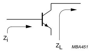
Fig.16 Definition of transistor impedance.
