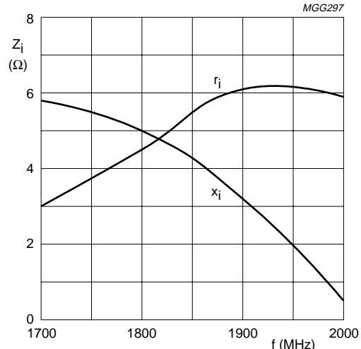
$V_{CE} = 26$  V;  $I_{CQ} = 80$  mA;  $P_L = 30$  W;  $T_{mb} = 25$  °C.
