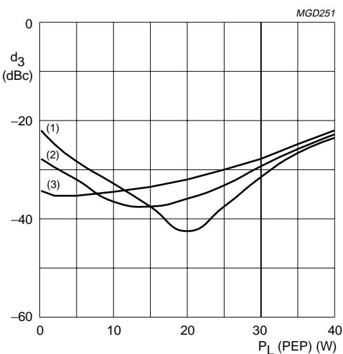
$V_{CE} = 26$  V;  $f_1 = 1950$  MHz;  $f_2 = 1950.1$  MHz.
