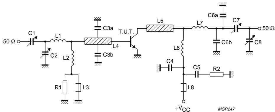
Fig.8 Class-B test circuit at  $f = 175$  MHz.
