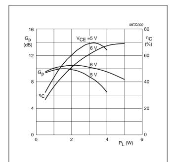
Pulsed, class-AB; f = 900 MHz;  $I_{\rm CQ}$  = 2 mA; tuned at P  $_{\rm L}$  = 3.5 W;  $T_{\rm s}$   $\leq$  60 °C.
