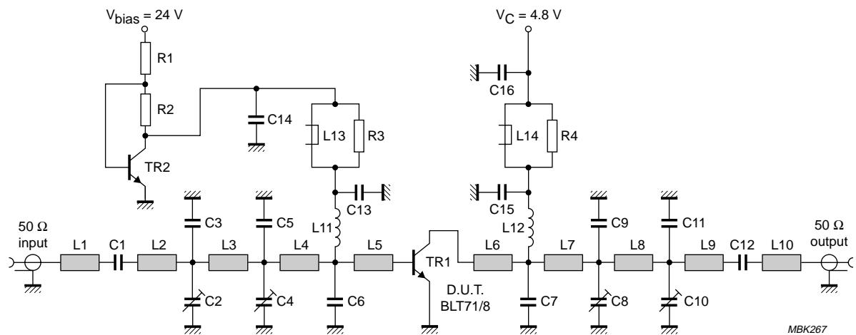
Fig.6 Class-AB test circuit at  $f = 900\text{ MHz}$ .
