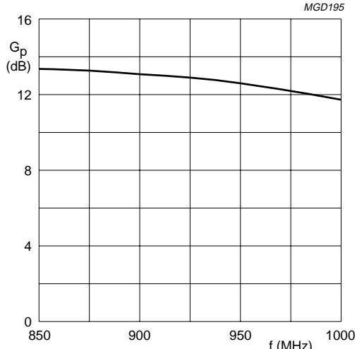
$V_{CE} = 4.8$  V;  $I_{CQ} = 3$  mA;  $P_L = 1.2$  W;  $T_{amb} = 25$  °C.
