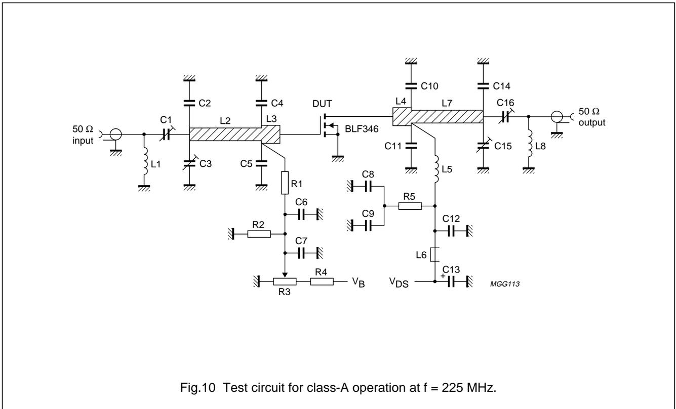
Fig.10 Test circuit for class-A operation at f = 225 MHz.
