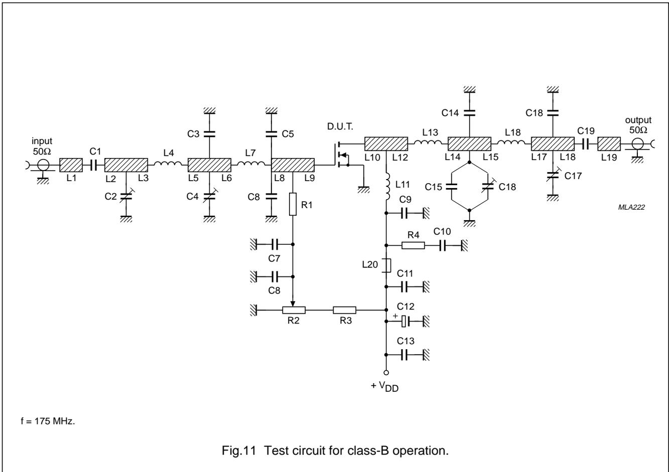
Fig.11 Test circuit for class-B operation.
