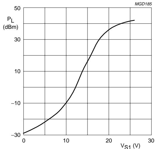
$f = 940$  MHz;  $V_{S2} = 26$  V;  $Z_S = Z_L = 50 \Omega$ ;  $T_{mb} = 25$  °C.
