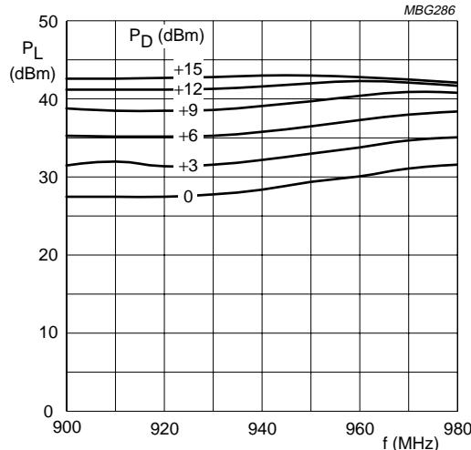
$V_{S1} = V_{S2} = 26$  V;  $Z_S = Z_L = 50 \Omega$ ;  $T_{mb} = 25$  °C.
