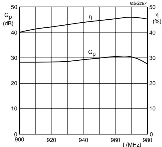
$V_{S1} = V_{S2} = 26$  V;  $P_L = 16$  W;  $Z_S = Z_L = 50 \Omega$ ;  $T_{mb} = 25$  °C.
