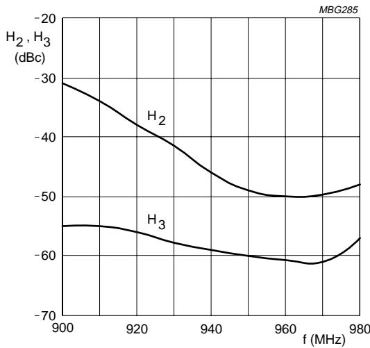
$V_{S1} = V_{S2} = 26$  V;  $P_L = 16$  W;  $Z_S = Z_L = 50 \Omega$ ;  $T_{mb} = 25$  °C.
