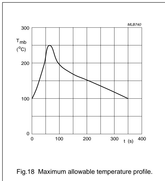
Fig.18 Maximum allowable temperature profile.
