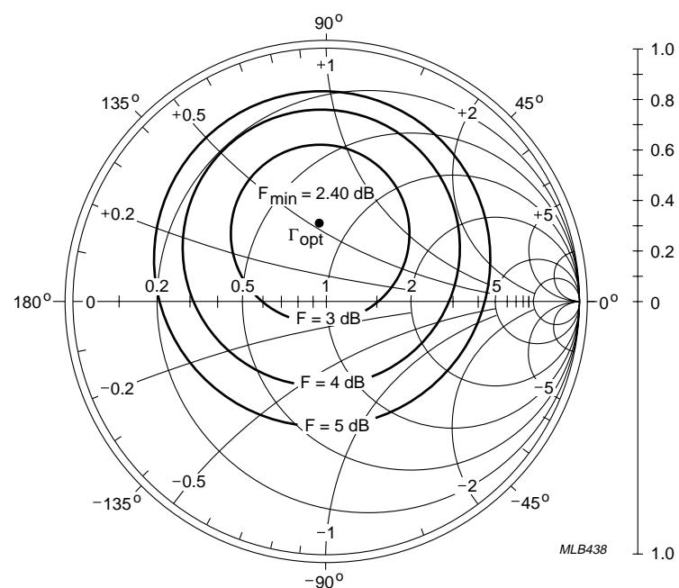
$V_{CE} = -5$  V;  $I_C = -10$  mA;  $f = 500$  MHz;  $Z_0 = 50 \Omega$ .
