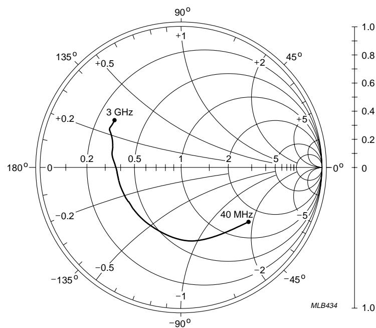
$V_{CE} = -10 \text{ V}; I_C = -30 \text{ mA}.$ Fig.10 Common emitter input reflection coefficient ( $s_{11}$ ), typical values.
