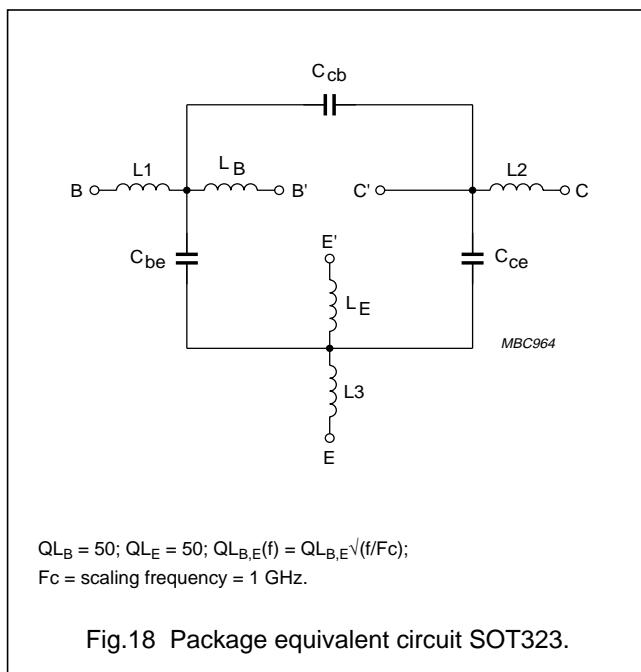
Fig.18 Package equivalent circuit SOT323.
