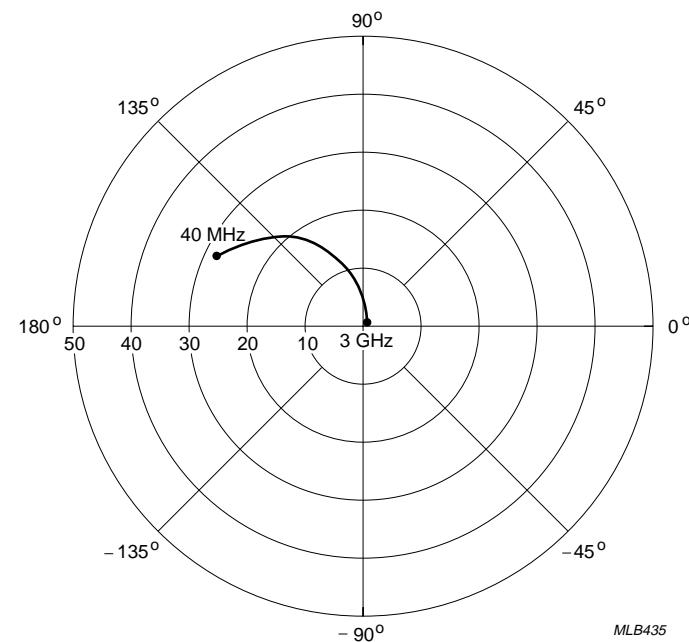
$V_{CE} = -10 \text{ V}; I_C = -30 \text{ mA}.$ Fig.11 Common emitter forward transmission coefficient ( $s_{21}$ ), typical values.
