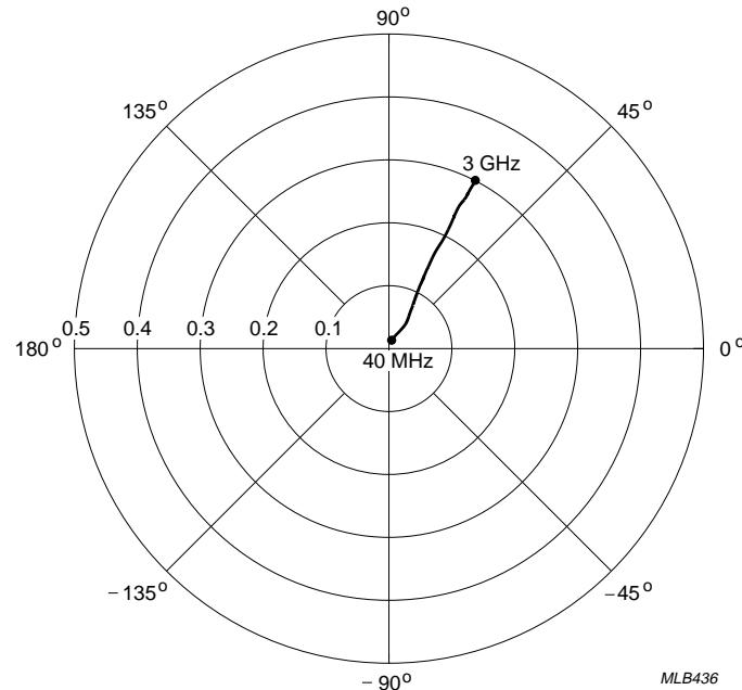
$V_{CE} = -10 \text{ V}; I_C = -30 \text{ mA.}$ Fig.12 Common emitter reverse transmission coefficient ( $s_{12}$ ), typical values.
