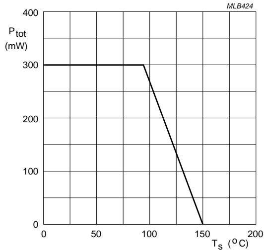
Fig.2 Power derating as a function of the soldering point temperature.
