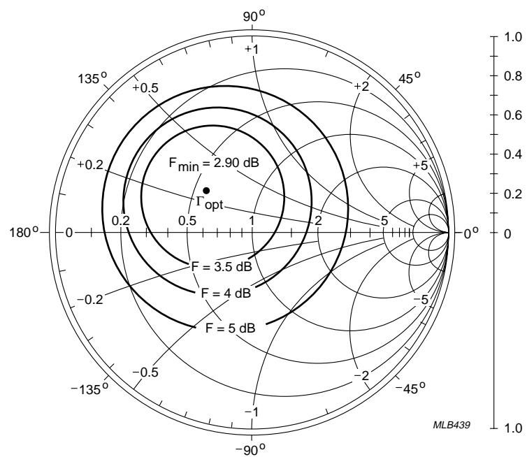
$V_{CE} = -5$  V;  $I_C = -10$  mA;  $f = 1$  GHz;  $Z_0 = 50 \Omega$ .
