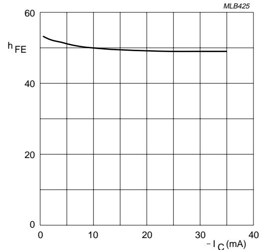
$V_{CE} = -5$  V;  $T_j = 25$   $^{\circ}$ C.
