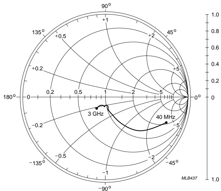
$V_{CE} = -10 \text{ V}; I_C = -30 \text{ mA.}$ Fig.13 Common emitter output reflection coefficient ( $s_{22}$ ), typical values.
