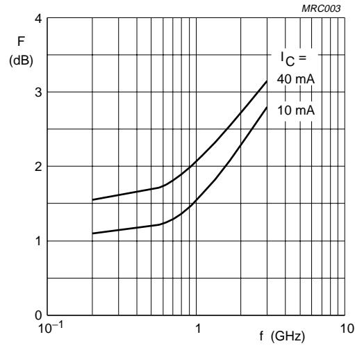
$V_{CE} = 8 \text{ V}; T_{amb} = 25^\circ\text{C}.$
