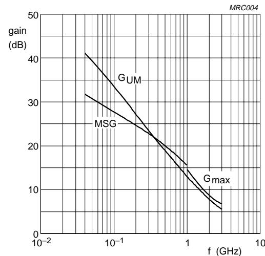
$I_C = 10\text{ mA}; V_{CE} = 8\text{ V}; T_{amb} = 25^\circ\text{C}$ .
