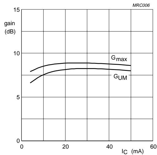
Fig.7 Gain as a function of collector current.
