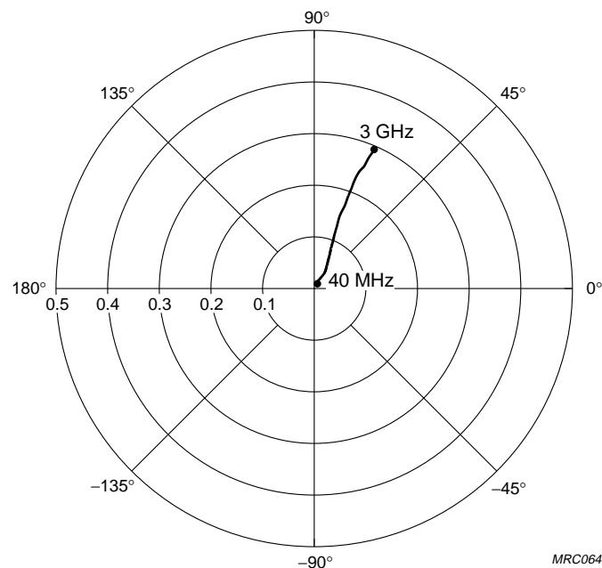
$I_C = 40 \text{ mA}; V_{CE} = 8 \text{ V}.$ Fig.16 Common emitter reverse transmission coefficient ( $s_{12}$ ).
