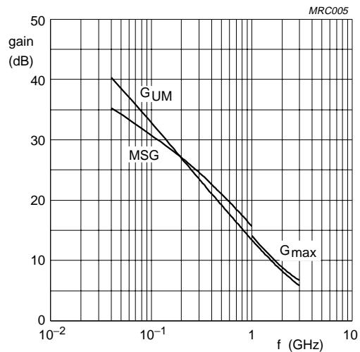
$I_C = 40\text{ mA}; V_{CE} = 8\text{ V}; T_{amb} = 25^\circ\text{C}$ .
