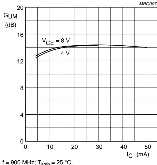
Fig.6 Maximum unilateral power gain as a function of collector current.
