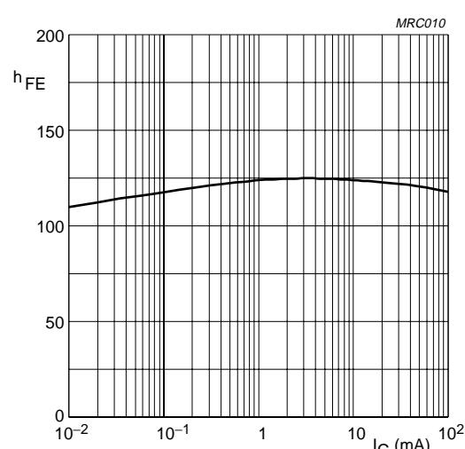
$V_{CE} = 8$  V;  $T_j = 25$   $^{\circ}$ C.
