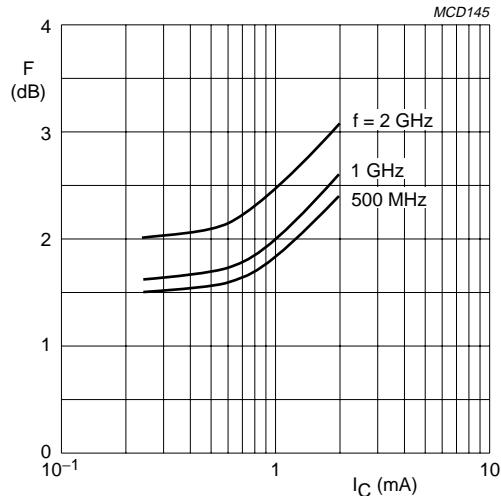
$V_{CE} = 1 \text{ V}; T_{amb} = 25 \text{ }^{\circ}\text{C}.$
