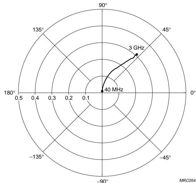
$I_C = 1 \text{ mA}; V_{CE} = 1 \text{ V}.$ Fig.17 Common emitter reverse transmission coefficient ( $S_{12}$ ).
