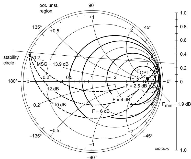
$I_C = 1 \text{ mA}; V_{CE} = 1 \text{ V}; f = 500 \text{ MHz}; Z_o = 50 \Omega.$
