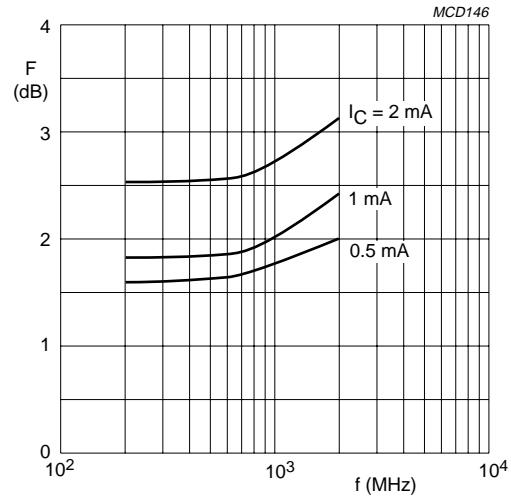
$V_{CE} = 1 \text{ V}; T_{amb} = 25 \text{ }^{\circ}\text{C}.$
