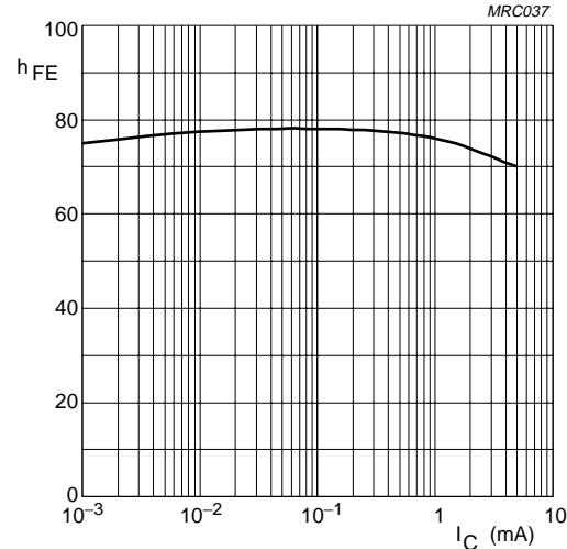
$V_{CE} = 1$  V;  $T_j = 25$   $^{\circ}$ C.
