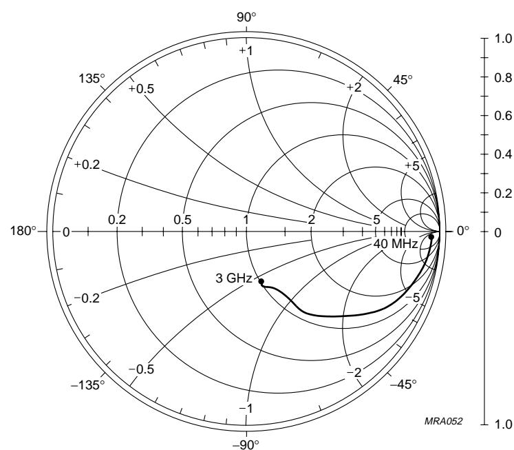
$I_C = 1 \text{ mA}$ ;  $V_{CE} = 1 \text{ V}$ ;
