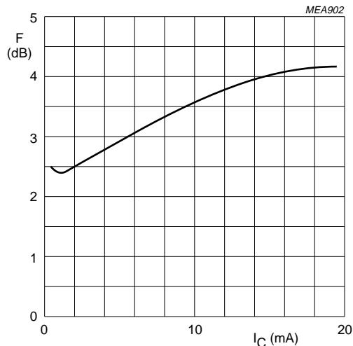
$V_{CE} = 5$  V;  $Z_s = 60$  Ω;  $f = 800$  MHz;  $T_{amb} = 25$  °C.
