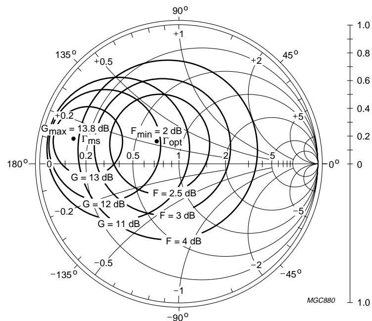
$f = 1 \text{ GHz}; V_{CE} = 8 \text{ V}; I_C = 10 \text{ mA}; Z_o = 50 \Omega.$
