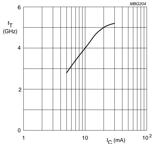
$V_{CE} = 5$  V;  $f = 500$  MHz;  $T_{amb} = 25$  °C.
