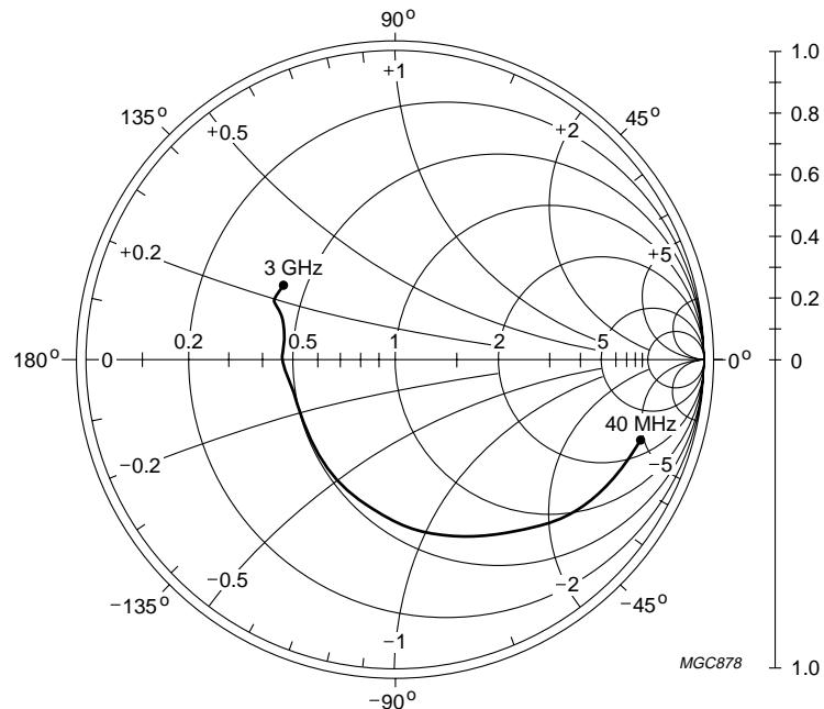
$V_{CE} = 8 \text{ V}; I_C = 30 \text{ mA}; Z_o = 50 \Omega.$ Fig.15 Common emitter input reflection coefficient ( $s_{11}$ ); typical values.
