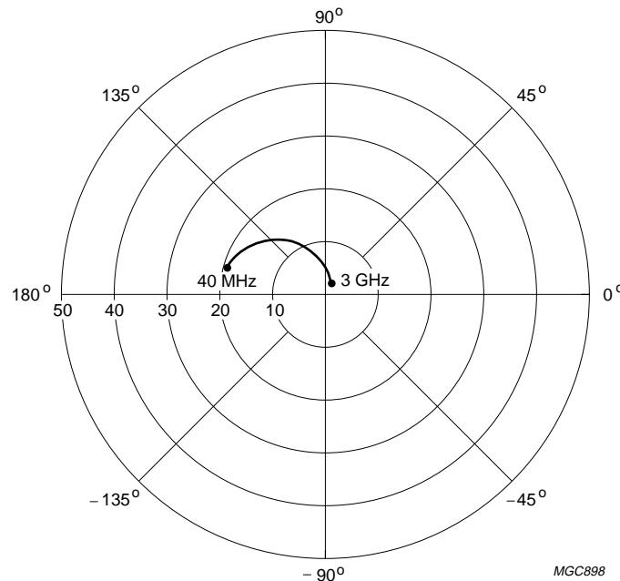
$V_{CE} = 8 \text{ V}; I_C = 30 \text{ mA}.$ Fig.16 Common emitter forward transmission coefficient ( $s_{21}$ ); typical values.
