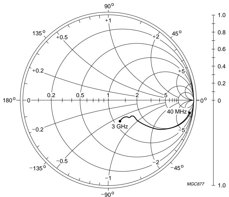
$V_{CE} = 8 \text{ V}; I_C = 30 \text{ mA}; Z_0 = 50 \Omega.$ Fig.18 Common emitter output reflection coefficient ( $s_{22}$ ); typical values.
