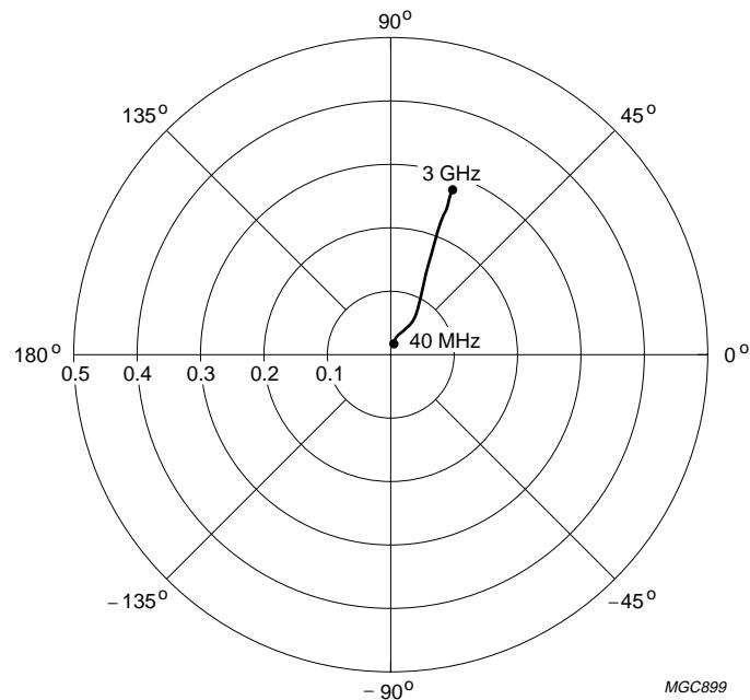
$V_{CE} = 8 \text{ V}; I_C = 30 \text{ mA}.$ Fig.17 Common emitter reverse transmission coefficient ( $s_{12}$ ); typical values.
