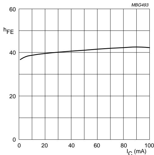
$V_{CE} = 10 \text{ V}; t_p = 500 \mu\text{s.}$
