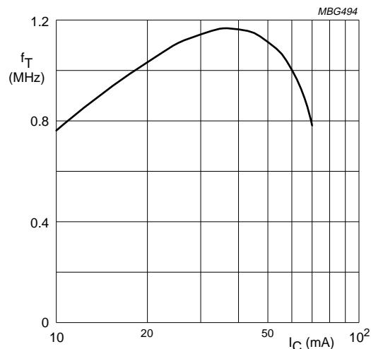
$V_{CE} = 10 \text{ V}; f = 500 \text{ MHz.}$
