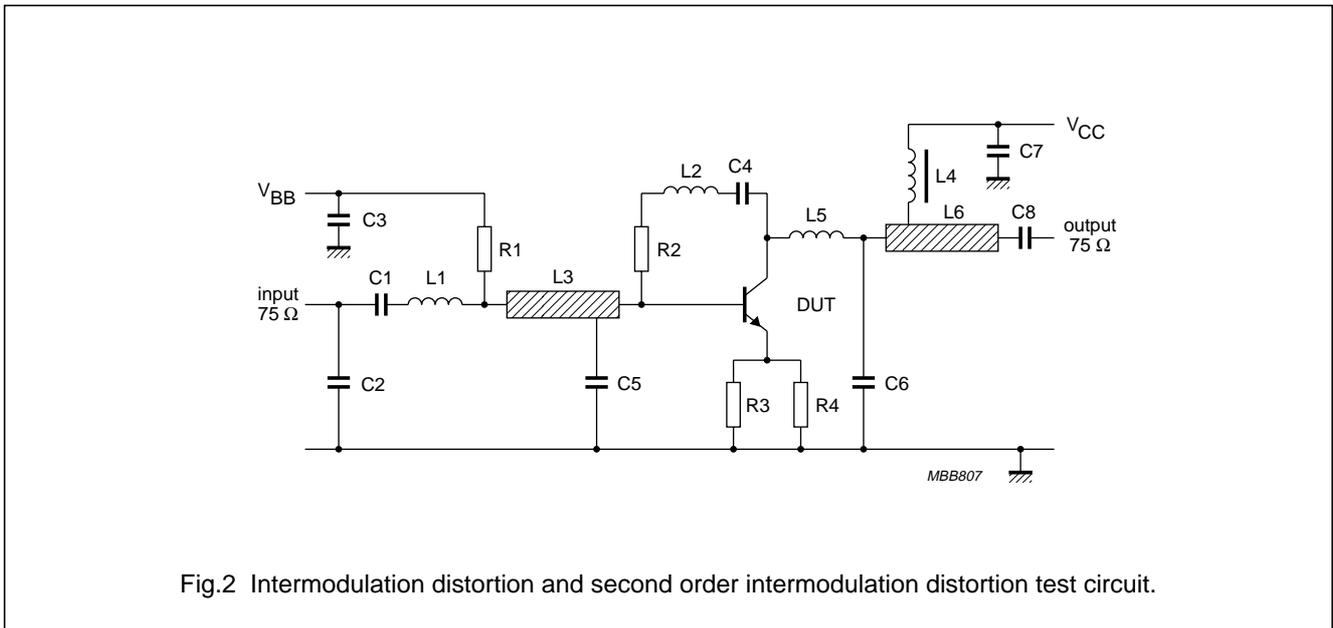
Fig.2 Intermodulation distortion and second order intermodulation distortion test circuit.
