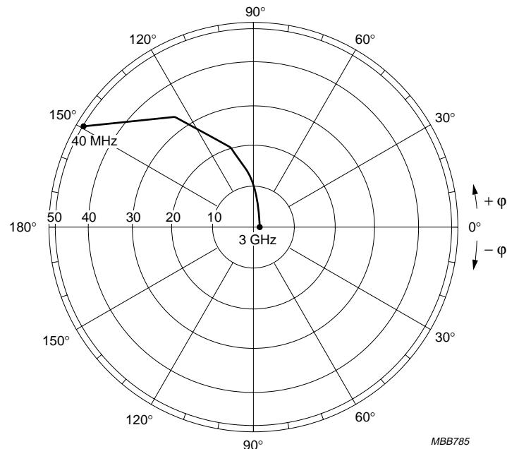
$I_C = 45 \text{ mA}; V_{CE} = 10 \text{ V.}$ Fig.19 Common emitter reverse transmission coefficient ( $S_{12}$ ).
