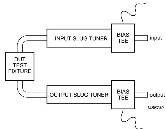
Fig.3 Measurement set-up for third order intercept point and 1 dB gain compression.
