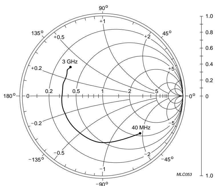
$V_{CE} = 8 \text{ V}; I_C = 40 \text{ mA}; Z_o = 50 \Omega.$ Fig.19 Common emitter input reflection coefficient ( $s_{11}$ ); typical values.
