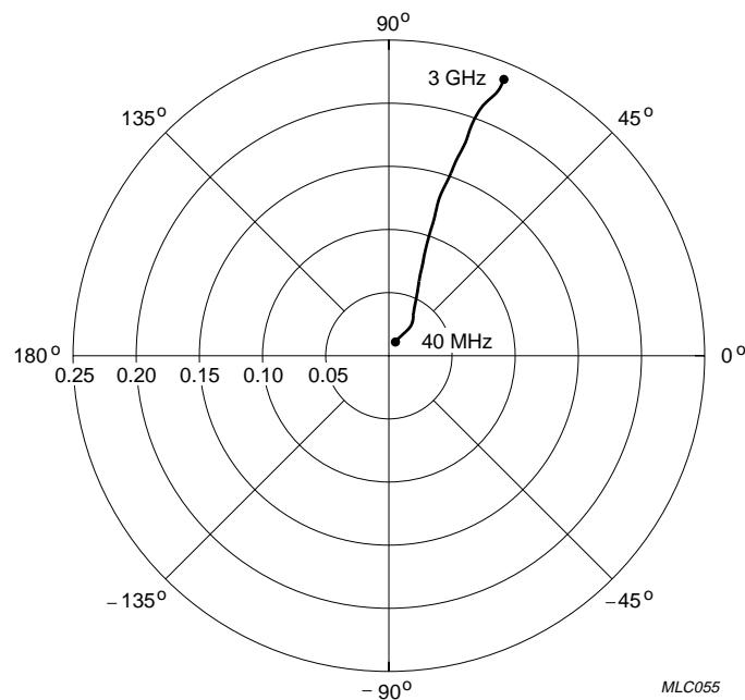
$V_{CE} = 8 \text{ V}; I_C = 40 \text{ mA}.$ Fig.21 Common emitter reverse transmission coefficient ( $S_{12}$ ); typical values.
