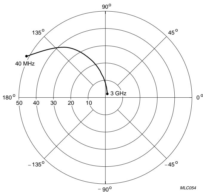
$V_{CE} = 8 \text{ V}; I_C = 40 \text{ mA}.$ Fig.20 Common emitter forward transmission coefficient ( $s_{21}$ ); typical values.
