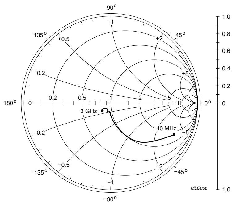
$V_{CE} = 8 \text{ V}; I_C = 40 \text{ mA}; Z_o = 50 \Omega.$ Fig.22 Common emitter output reflection coefficient ( $S_{22}$ ); typical values.
