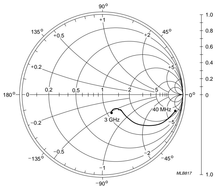
$V_{CE} = 6 \text{ V}; I_C = 20 \text{ mA}; Z_o = 50 \Omega.$ Fig.21 Common emitter output reflection coefficient ( $S_{22}$ ); typical values.
