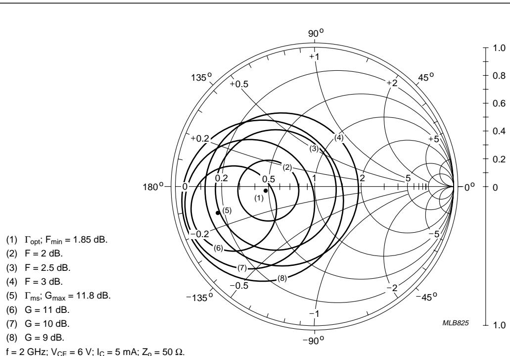
Fig.17 Common emitter noise figure circles; typical values.
