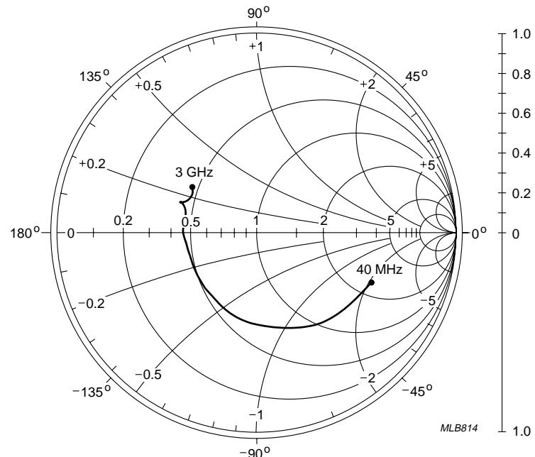
$V_{CE} = 6 \text{ V}; I_C = 20 \text{ mA}; Z_0 = 50 \Omega$ .Fig.18 Common emitter input reflection coefficient ( $S_{11}$ ); typical values.
