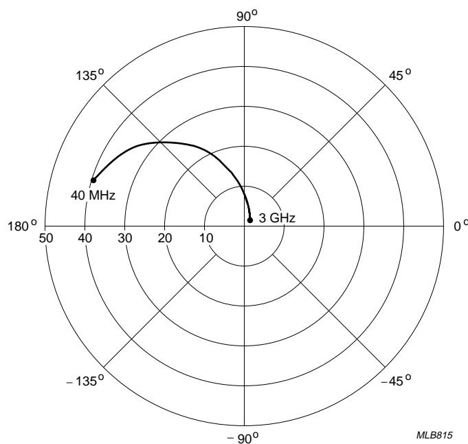
$V_{CE} = 6 \text{ V}; I_C = 20 \text{ mA}$ .Fig.19 Common emitter forward transmission coefficient ( $S_{21}$ ); typical values.
