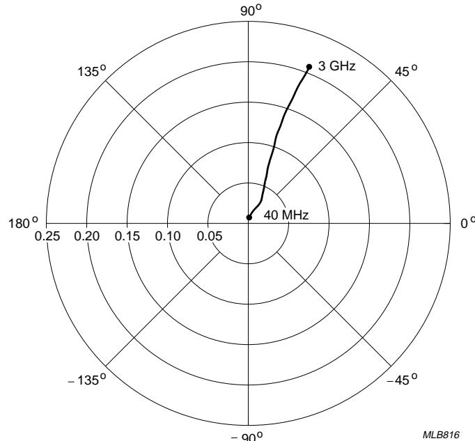
$V_{CE} = 6 \text{ V}; I_C = 20 \text{ mA}.$ Fig.20 Common emitter reverse transmission coefficient ( $S_{12}$ ); typical values.
