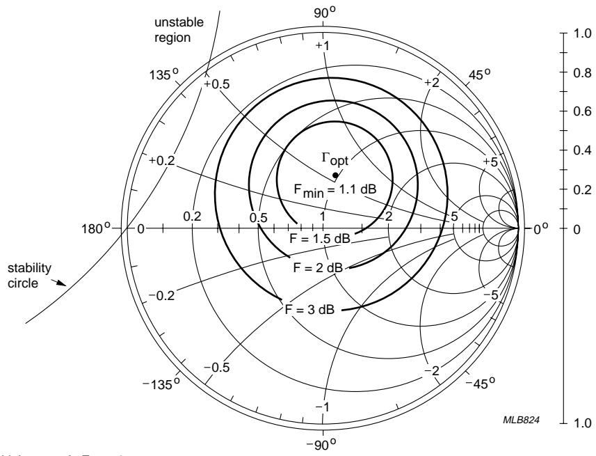
Fig.16 Common emitter noise figure circles; typical values.
