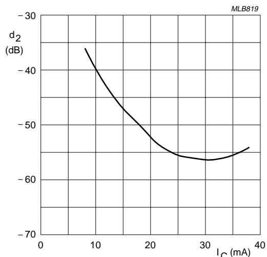
$V_o = 75$  mV;  $f_p + f_0 = 810$  MHz;  $V_{CE} = 6$  V;
