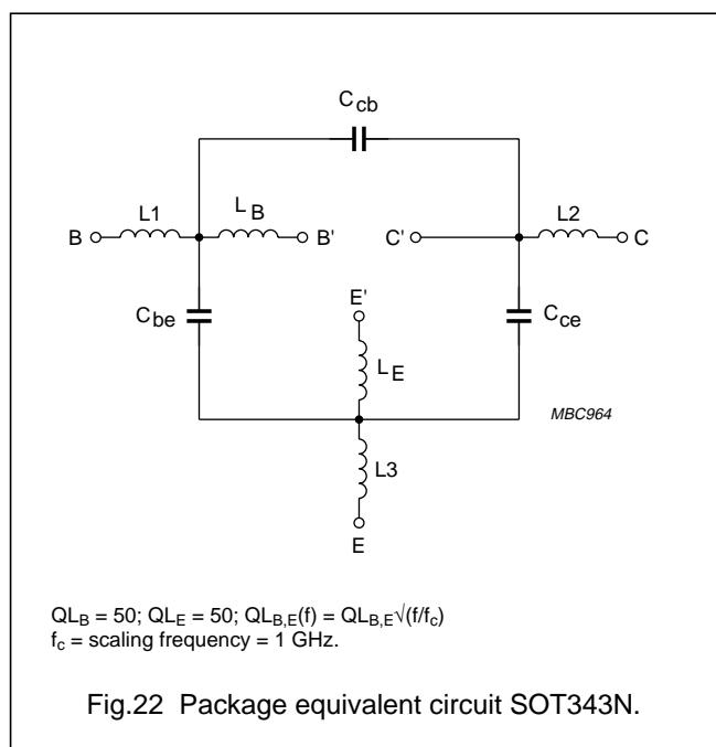
Fig.22 Package equivalent circuit SOT343N.
