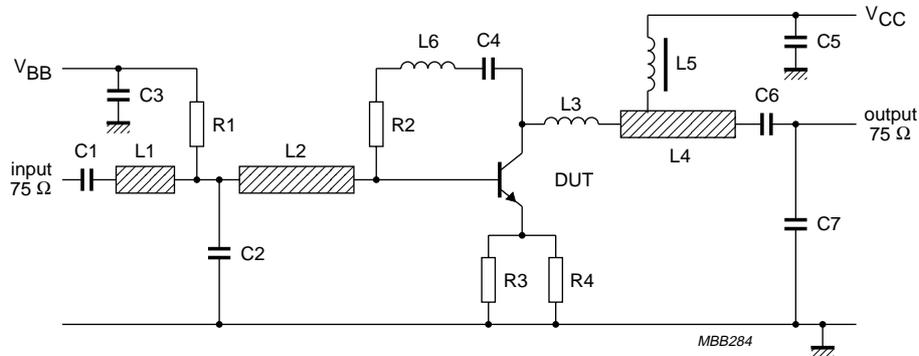
Fig.2 Intermodulation and second harmonic test circuit.
