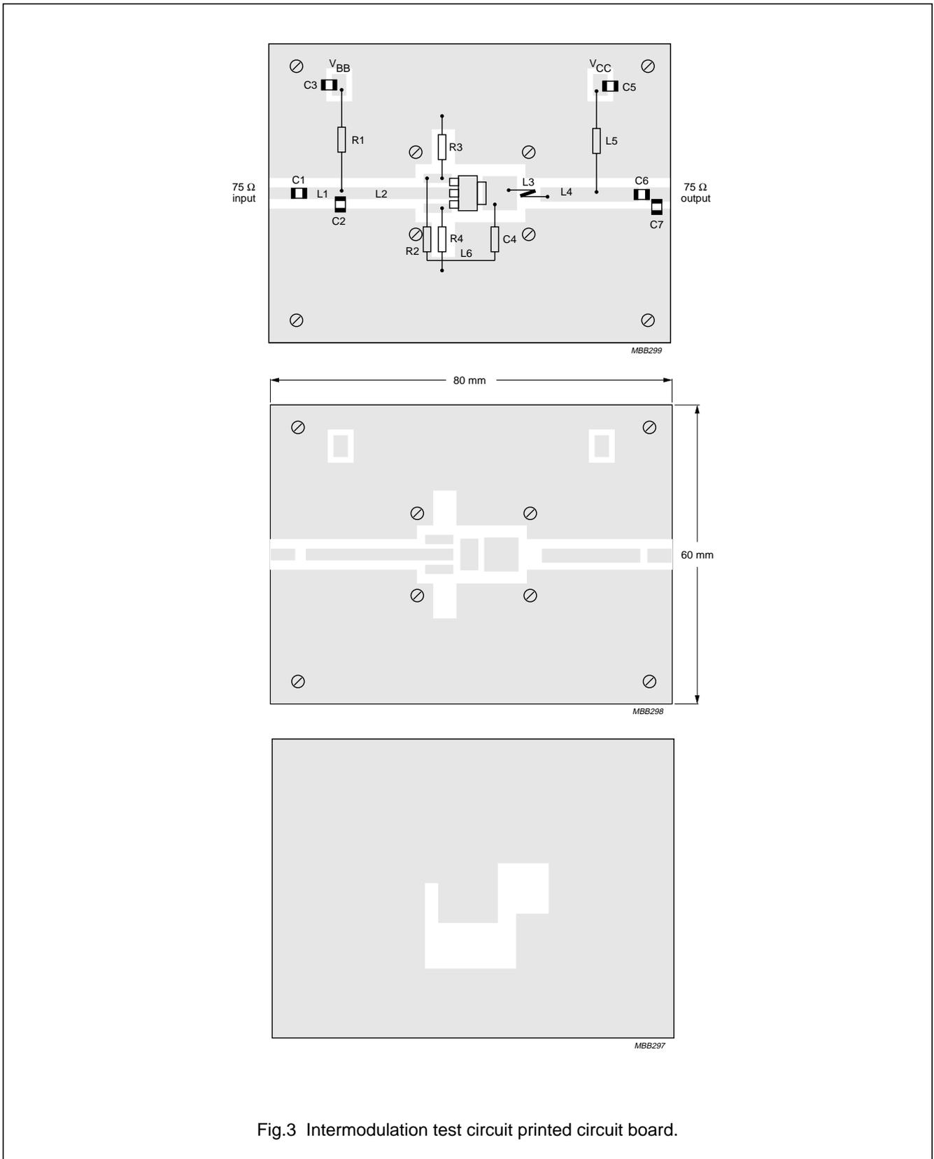
Fig.3 Intermodulation test circuit printed circuit board.
