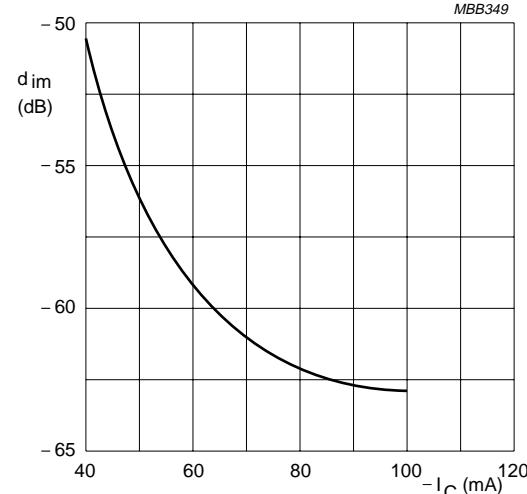
$V_{CE} = -10$  V;  $V_o = 550$  mV;  $T_{amb} = 25$  °C;
