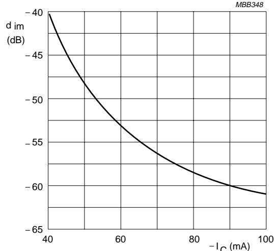
$V_{CE} = -10$  V;  $V_o = 650$  mV;  $T_{amb} = 25$  °C;
