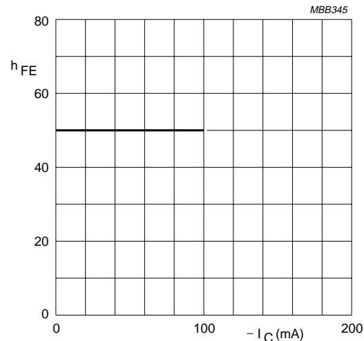
$V_{CE} = -10$  V;  $T_{amb} = 25$   $^{\circ}$ C.
