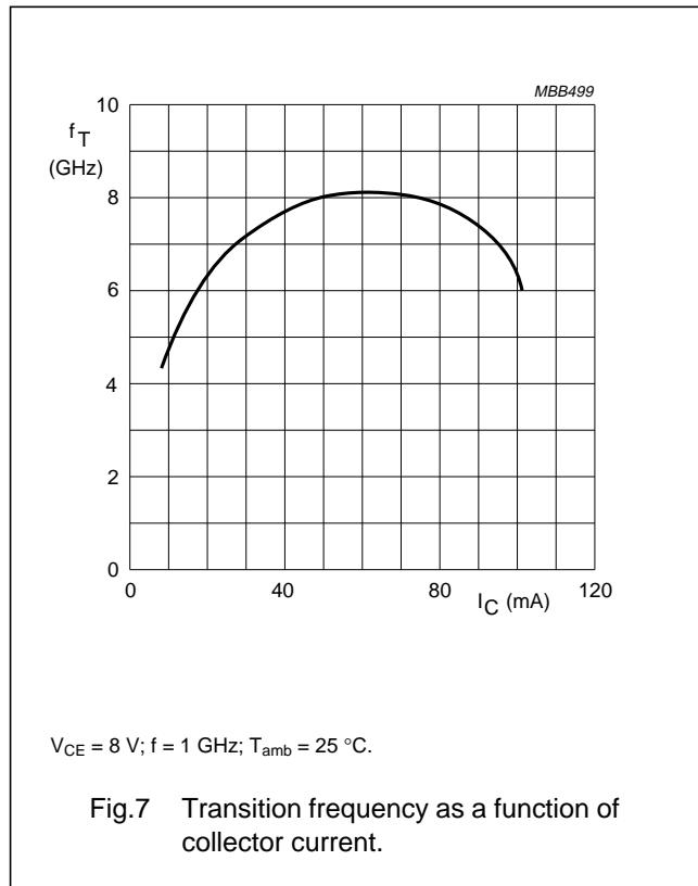
Fig.7 Transition frequency as a function of collector current.
