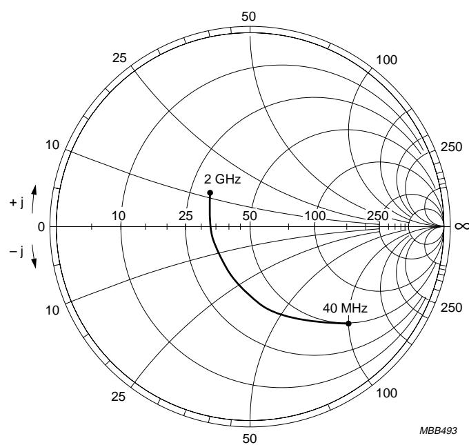
$I_C = 50 \text{ mA}; V_{CE} = 8 \text{ V}; T_{amb} = 25^\circ\text{C}; Z_0 = 50 \Omega.$
