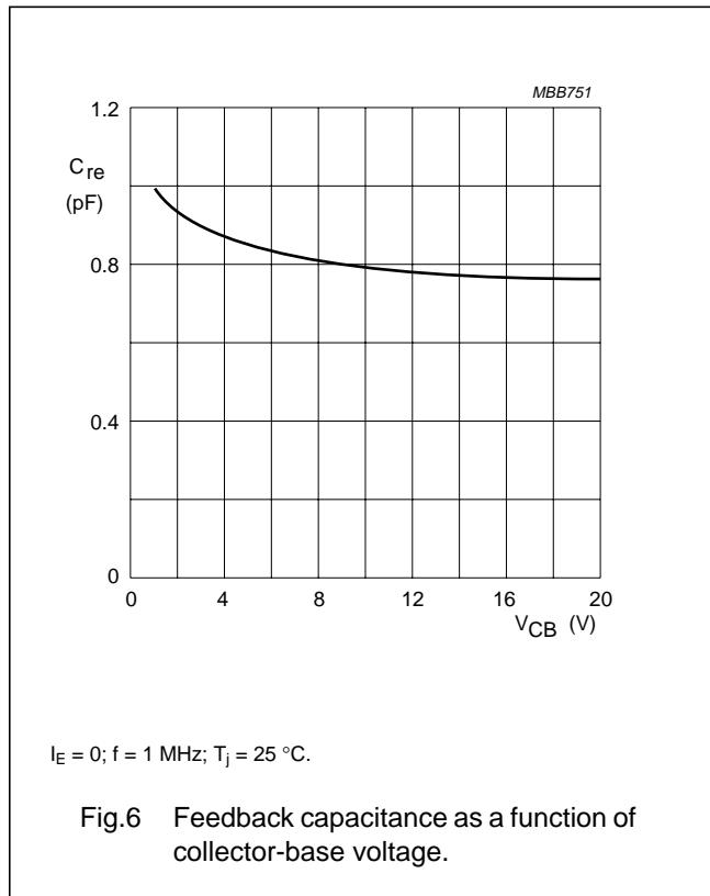
Fig.6 Feedback capacitance as a function of collector-base voltage.
