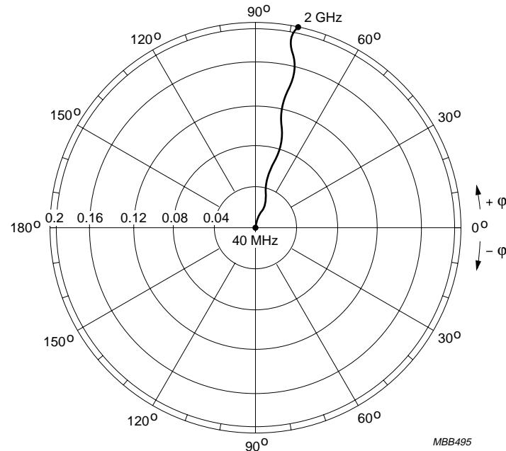
$I_C = 50 \text{ mA}; V_{CE} = 8 \text{ V}; T_{amb} = 25^\circ\text{C}.$
