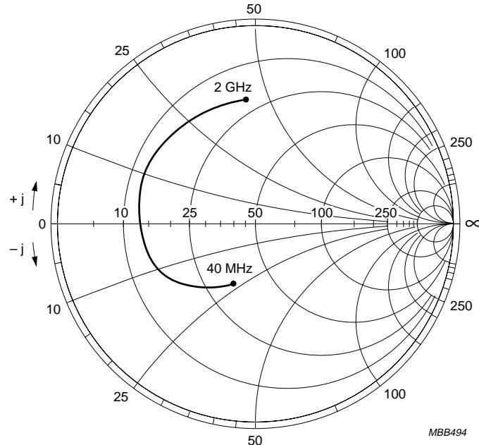
$I_C = 50 \text{ mA}; V_{CE} = 8 \text{ V}; T_{amb} = 25^\circ\text{C}; Z_0 = 50 \Omega.$ Fig.13 Common emitter input reflection coefficient ( $S_{11}$ ).
