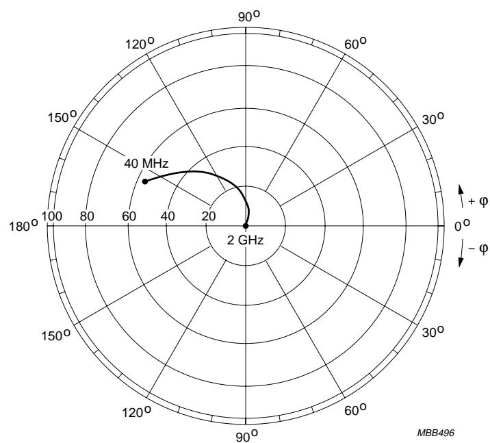
$I_C = 50 \text{ mA}; V_{CE} = 8 \text{ V}; T_{amb} = 25^\circ\text{C}.$ Fig.14 Common emitter forward transmission coefficient ( $S_{21}$ ).
