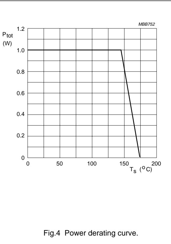
Fig.4 Power derating curve.
