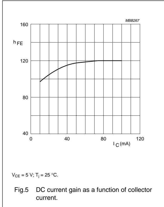
Fig.5 DC current gain as a function of collector current.
