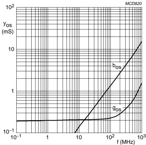
$V_{DS} = 8$  V;  $V_{GS} = 0$ ;  $T_{amb} = 25$  °C.
