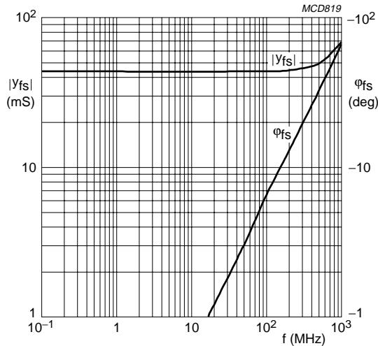
$V_{DS} = 8$  V;  $V_{GS} = 0$ ;  $T_{amb} = 25$  °C.
