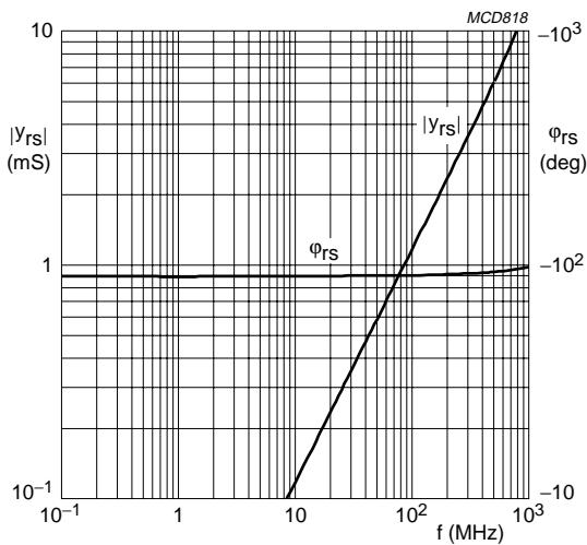
$V_{DS} = 5$  V;  $V_{G2} = 4$  V.
