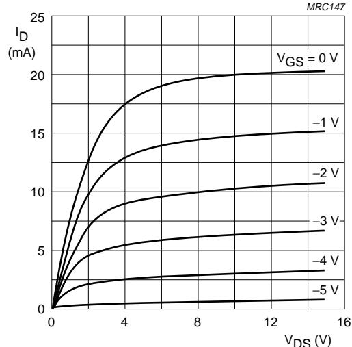
Fig.8 Typical output characteristics; BF556C.
