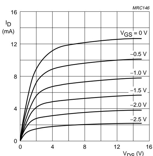
Fig.7 Typical output characteristics; BF556B.
