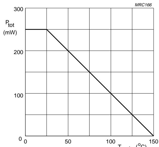
Fig.13 Power derating curve.
