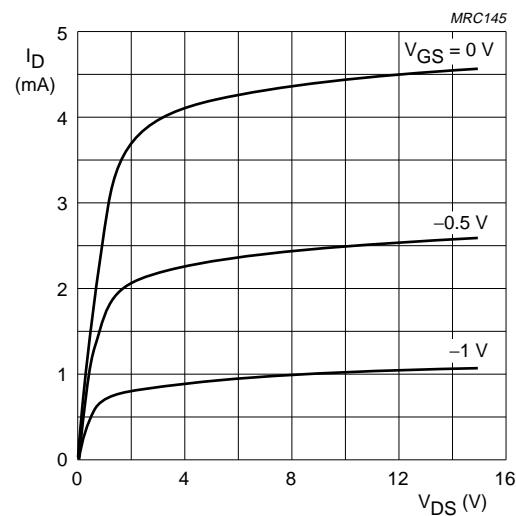
Fig.6 Typical output characteristics; BF556A.
