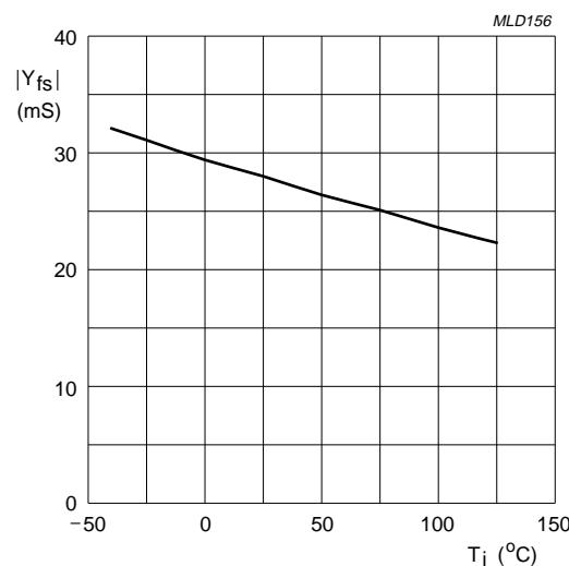
Fig.3 Forward transfer admittance as a function of junction temperature; typical values.
