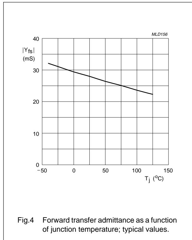
Fig.4 Forward transfer admittance as a function of junction temperature; typical values.
