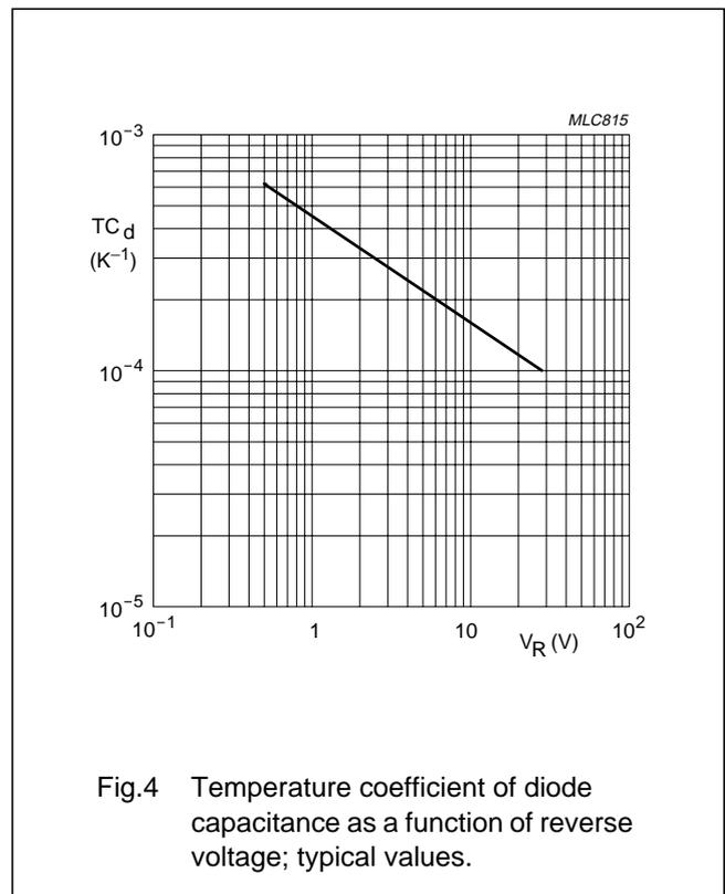
AM variable capacitance double diode
