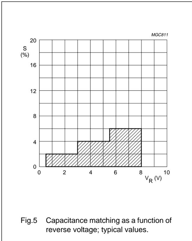
AM variable capacitance double diode
