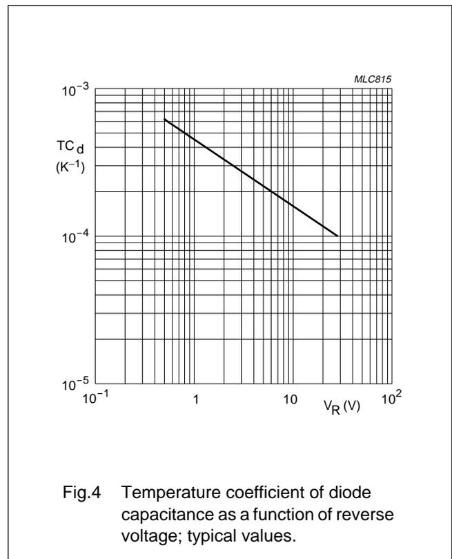
Variable capacitance diode
