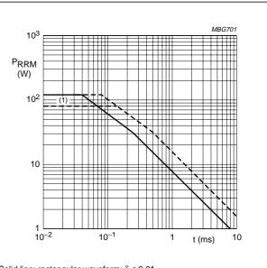
$\begin{array}{ll} \mbox{Solid line; rectangular waveform; $\delta \leq 0.01$.} \\ \mbox{Dotted line; triangular waveform; $\delta \leq 0.02$.} \\ \mbox{(1) Limited by } I_{RMM} = 600 \mbox{ mA}. \end{array}$
