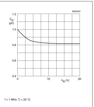
Diode capacitance as a function of reverse voltage; typical values.
