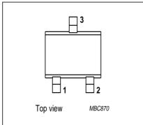
Fig.1 Simplified outline (SOT323) and pin configuration.
