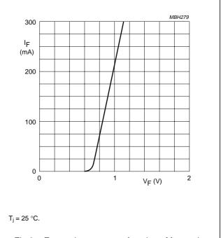
Fig.3 Forward current as a function of forward voltage; typical values.
