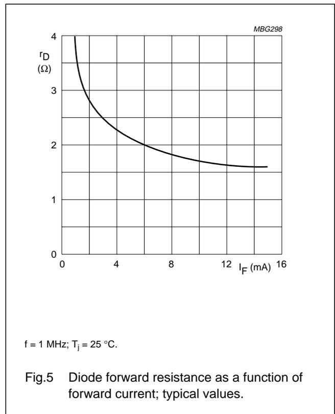
AM band-switching diode
