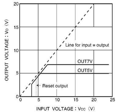
Fig.2 Input voltage vs. output voltage
