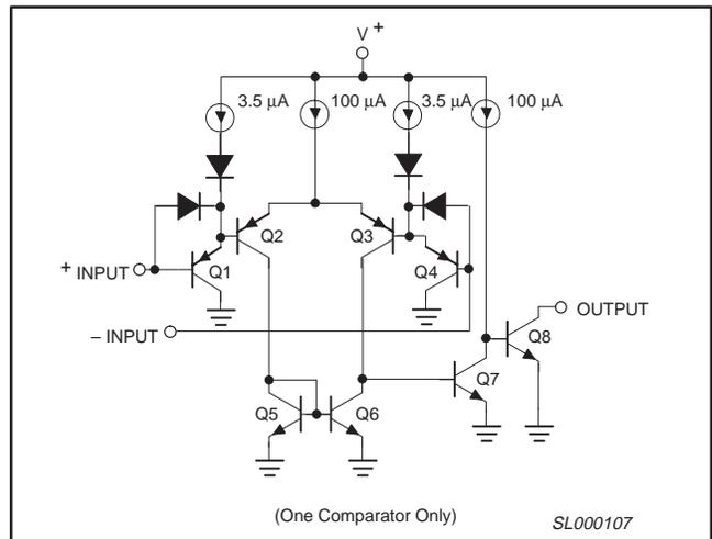
Figure 2. Equivalent Circuit
