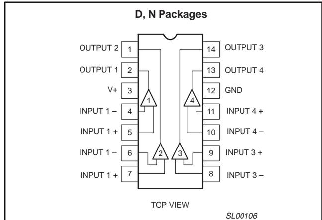
Figure 1. Pin Configuration
