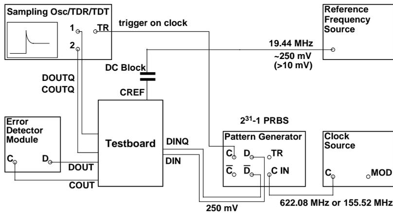
Above: Functional test setup: Data & Clock Recovery mode
