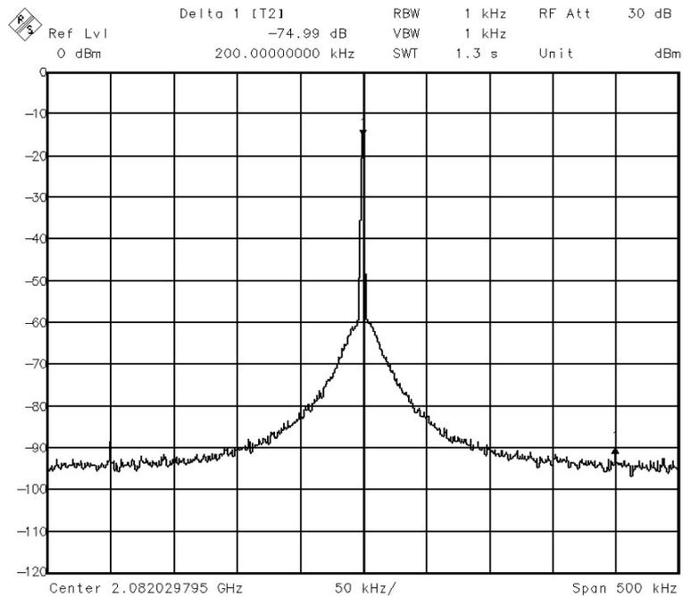
Fig. 35 - UMA1021M Synthesizer - Comparison Frequency Breakthrough (DCS Application).
