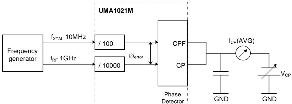
Fig. 8 - UMA1021M Principal Synthesizer Phase Detector Linearity Measurement.
