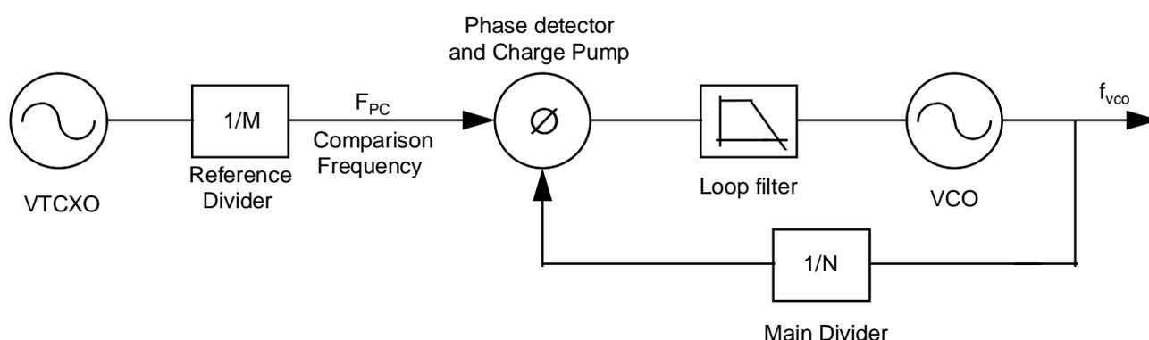
Fig. 25 - Basic Phase Lock Loop Block Diagram.
