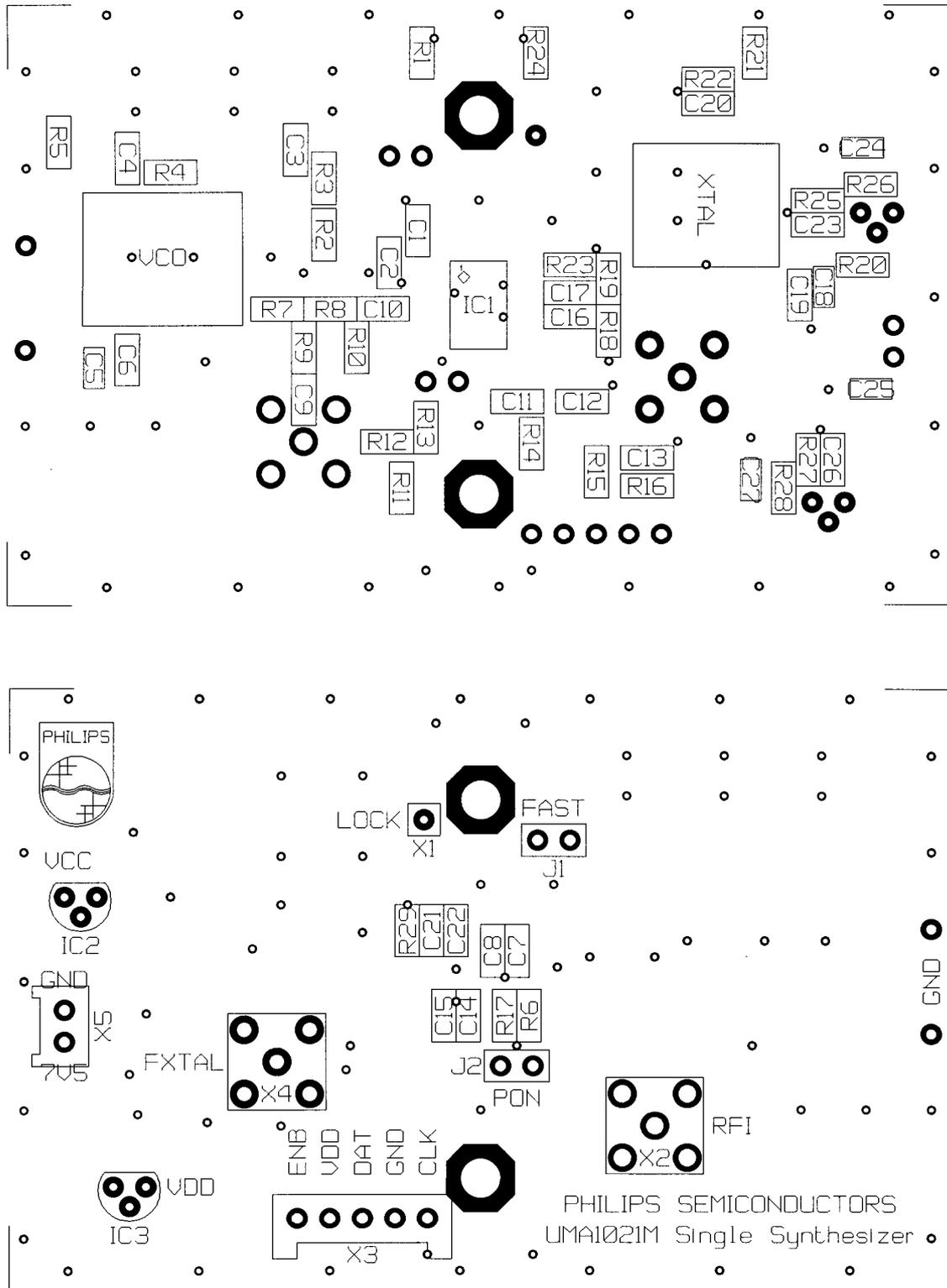
Fig. 48 - Demonstration Board Placement of Components.
