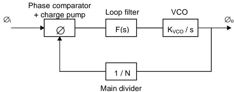
Fig. 45 - Block Diagram of a Phase Locked Loop.
