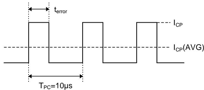
$$I_{CP}(AVG) = \left( \frac{t_{error}}{T_{PC}} \right) \times I_{CP}$$
