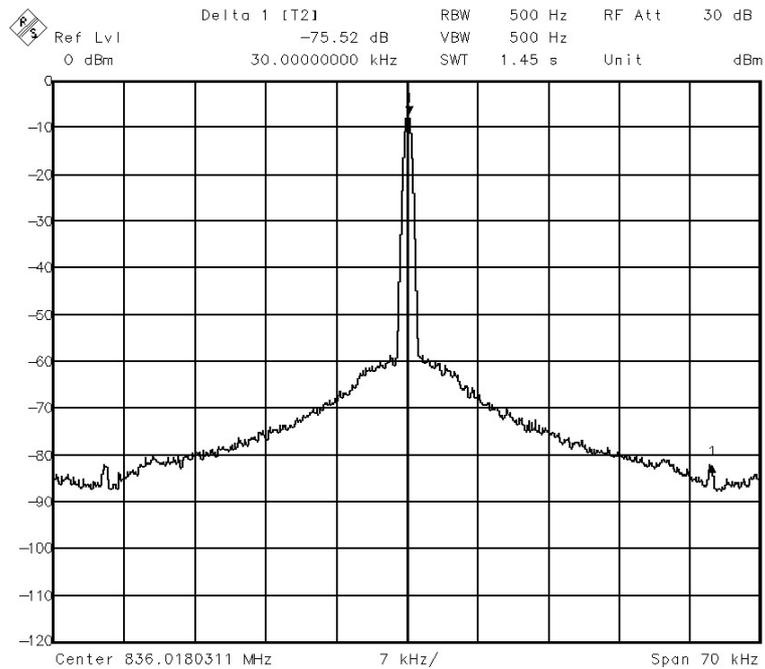
Fig. 41 - UMA1021M Synthesizer - Comparison Frequency Breakthrough (DAMPS Application).
