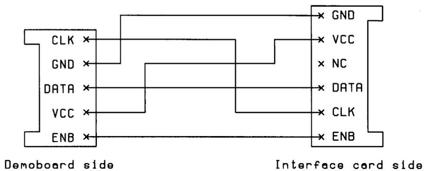
Fig. 49 - Interface Card pcb Layout and Cable Connection.
