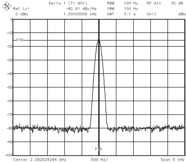
Fig. 34 - UMA1021M Synthesizer Output - Close in Noise (DCS Application).
