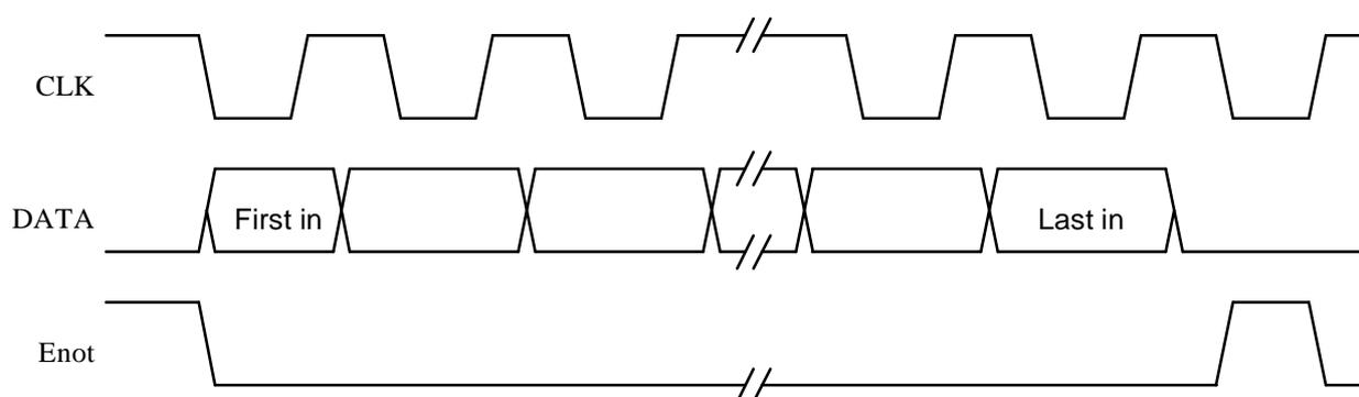
Fig. 17 - Serial Interface Timing Diagram.
