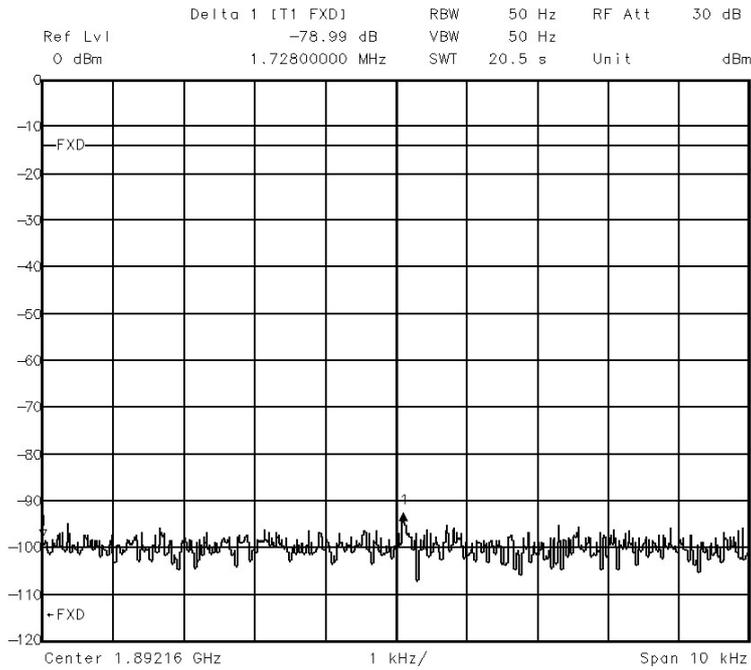
Fig. 39 - UMA1021M Synthesizer - Comparison Frequency Breakthrough (DECT Application).
