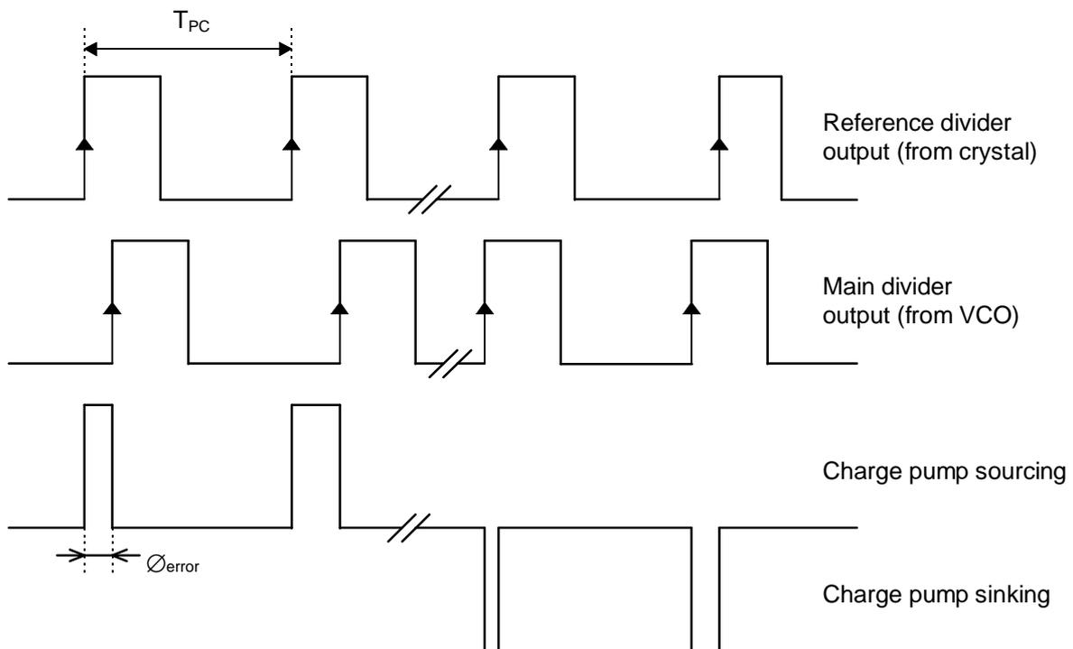
Fig. 3 - Principle of UMA1021M Phase Detector.
