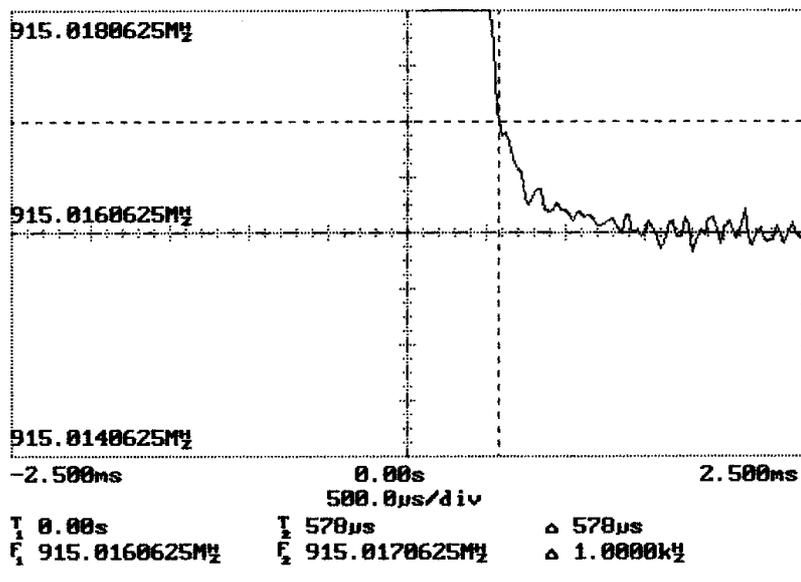
Fig. 32- Settling Time (890 to 915 MHz Step to Within 1 kHz).
