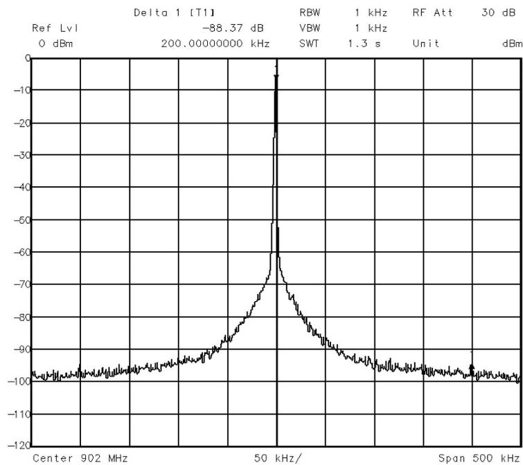
Fig. 31 - UMA1021M Synthesizer - Comparison Frequency Breakthrough (GSM Application).
