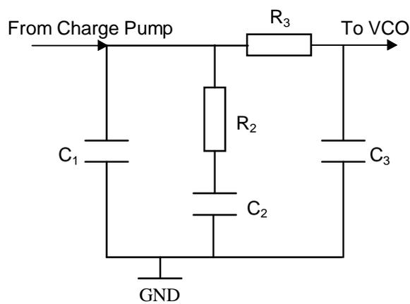
$$T_1 = (R_2 \times C_2 \times C_1) / (C_1 + C_2) ; T_2 = R_2 \times C_2 ; T_3 = R_3 \times C_3 \text{ if } C_2 \gg C_1 \gg C_3$$
