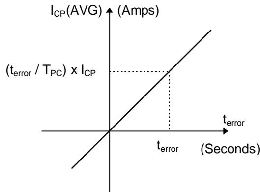
In order to find the real phase detector and charge pump gain for very small phase errors, we transform this curve by the equation: Phase Detector Gain (Amps/cycle) =  $I_{CP}(AVG) \times (T_{PC} / t_{error})$ . So the charge pump dynamic characteristics are obtained (see Fig. 10, Fig. 12, Fig. 14 and Fig. 16). Curves show measurements for source and sink gains.
