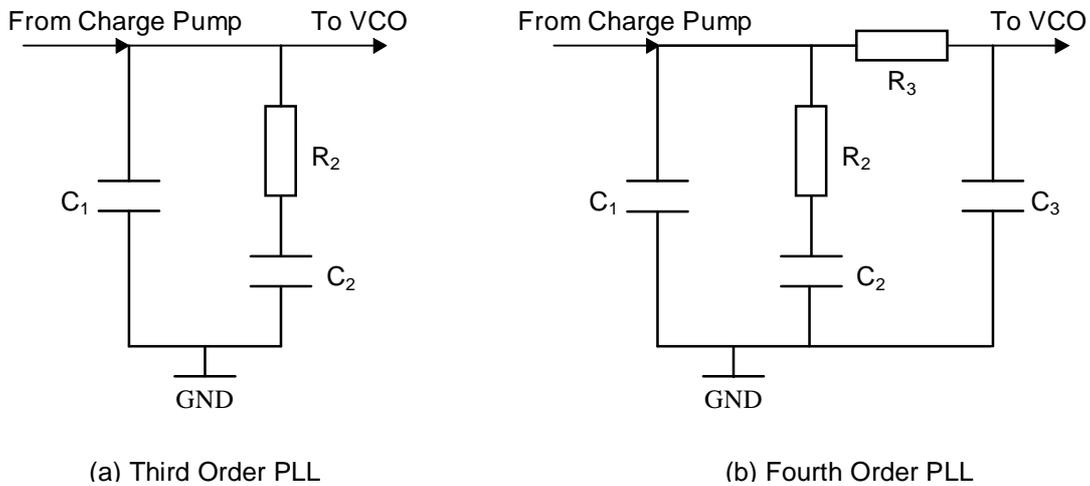
Fig. 26 - Different Types of Passive Loop Filter.
