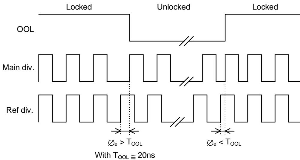
Fig. 24 - Operating Principle of the Out-Of-Lock Detector.
