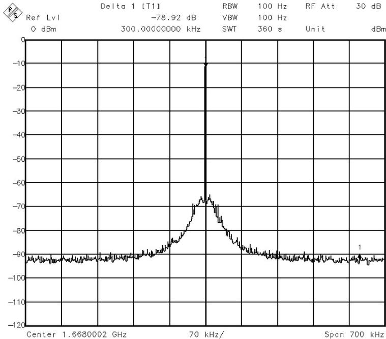
Fig. 37 - UMA1021M Synthesizer - Comparison Frequency Breakthrough (PHS Application).
