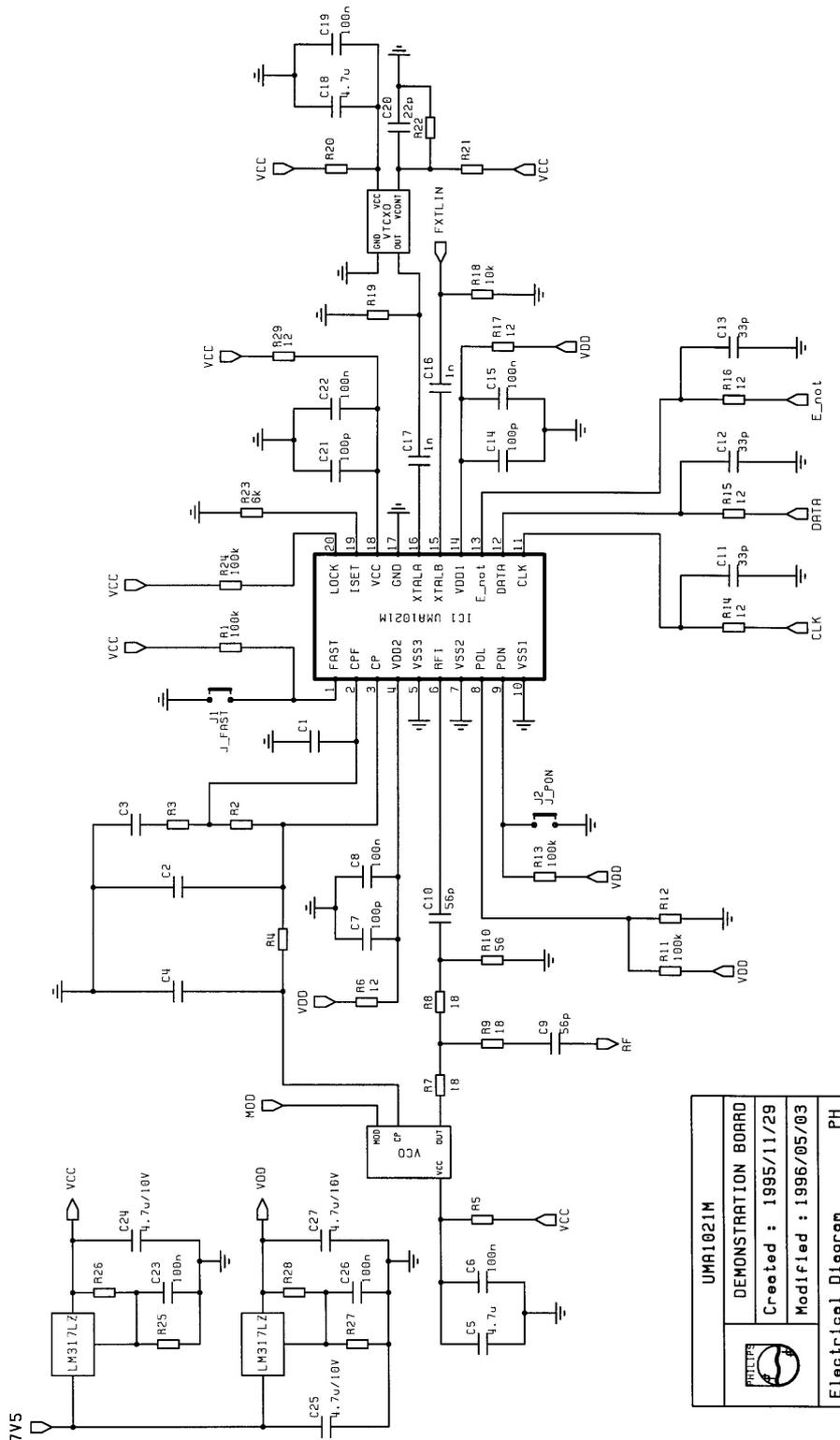
Fig. 46 - Demonstration Board Circuit Diagram.
