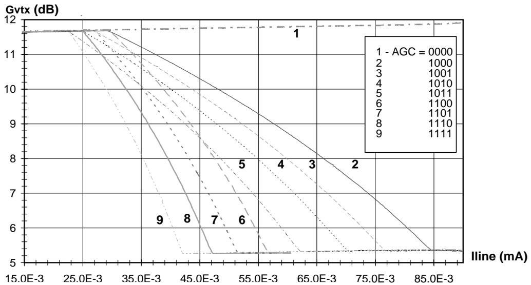
Fig.25 AGC control of the TX amplifier
