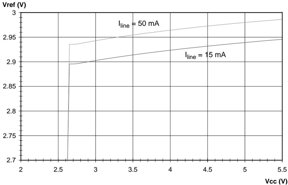
Fig.6 Dependency of V<sub>REF</sub> with the supply voltage V<sub>CC</sub>
