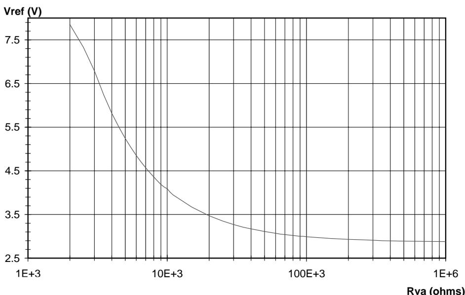
Fig.5 Adjustment of V<sub>REF</sub> with resistor R<sub>VA</sub>, connected between SLPE and REG
