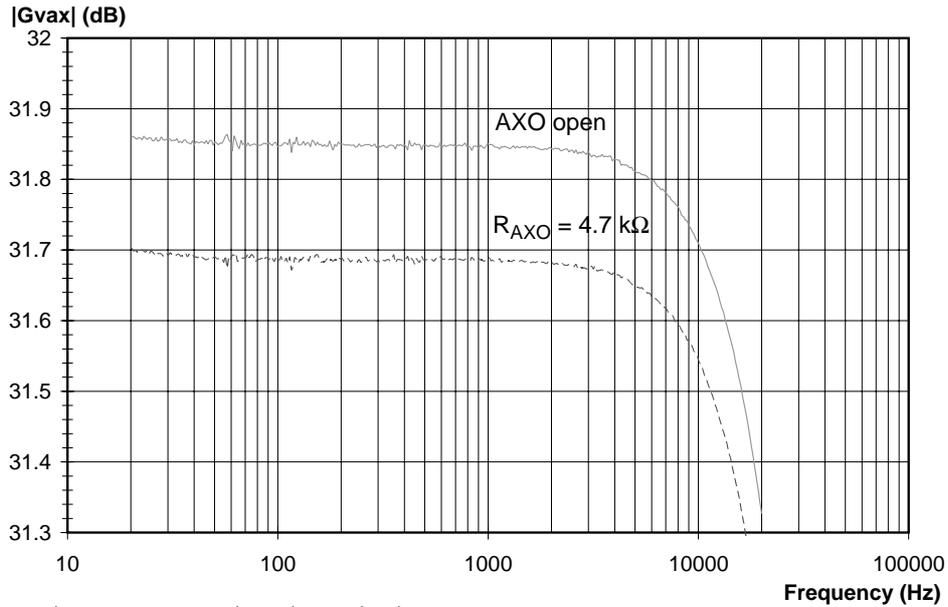
Fig.27 Gain of the auxiliary amplifier
