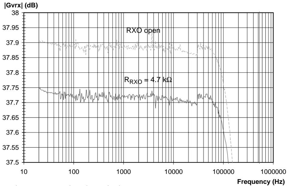
Fig.23 Gain of the receive amplifier
