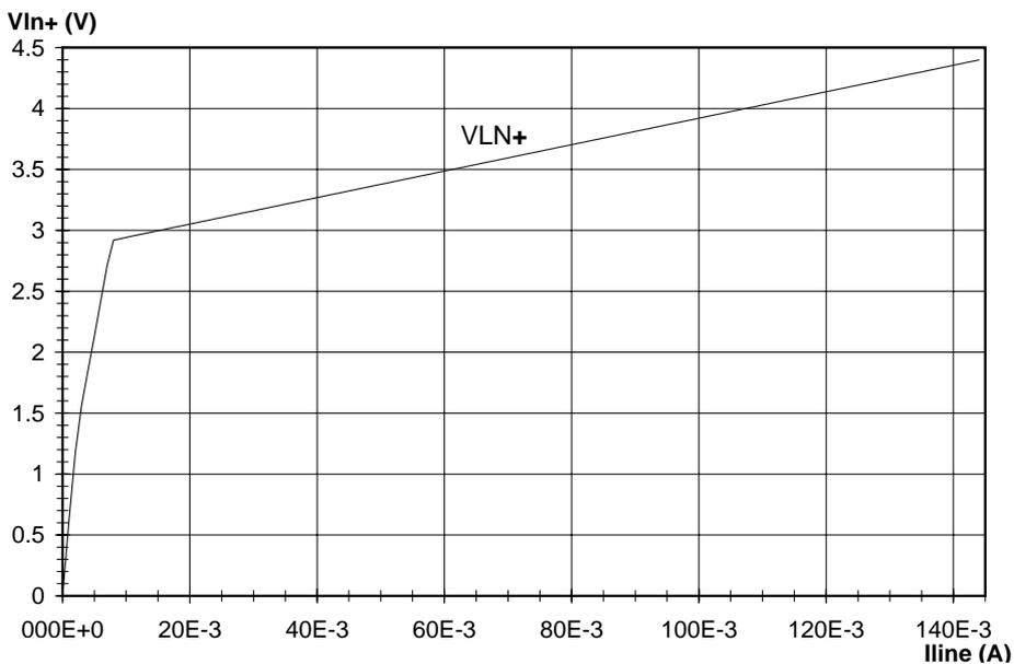
Fig.7 The voltage between VLN+ and GND versus I<sub>line</sub> at VRM
