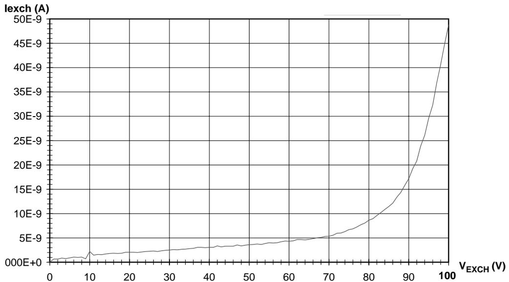
Fig.11 Leakage (line) current at on-hook conditions
