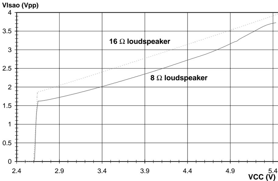
Fig.32 Output voltage capability of the loudspeaker amplifier
