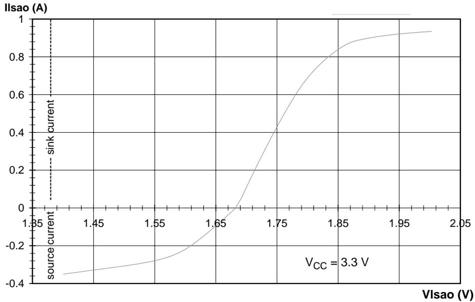
Fig.33 Output current capability at  $V_{CC} = 3.3$  V
