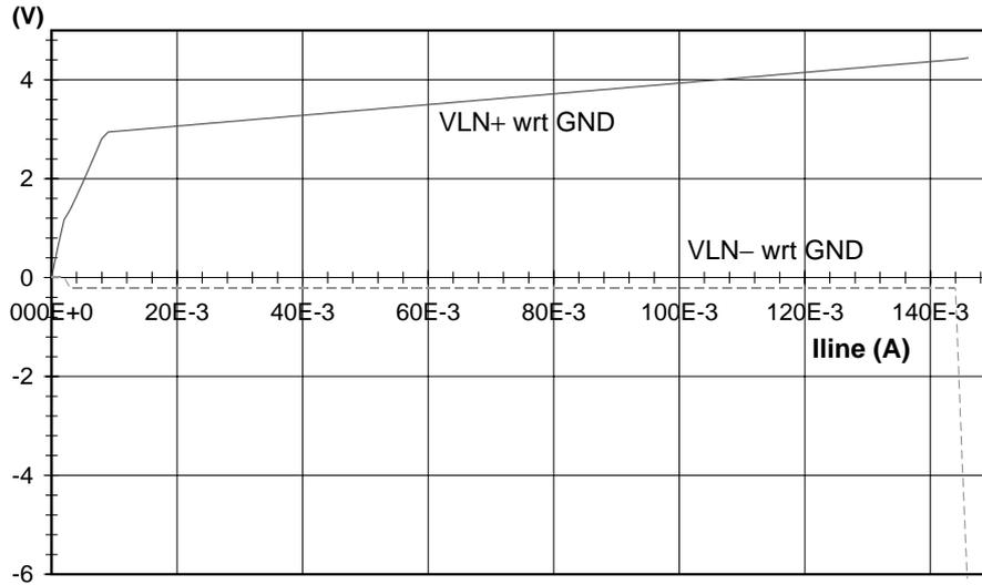
Fig.10 Activated current protection at  $I_{line} > 144 \text{ mA}$
