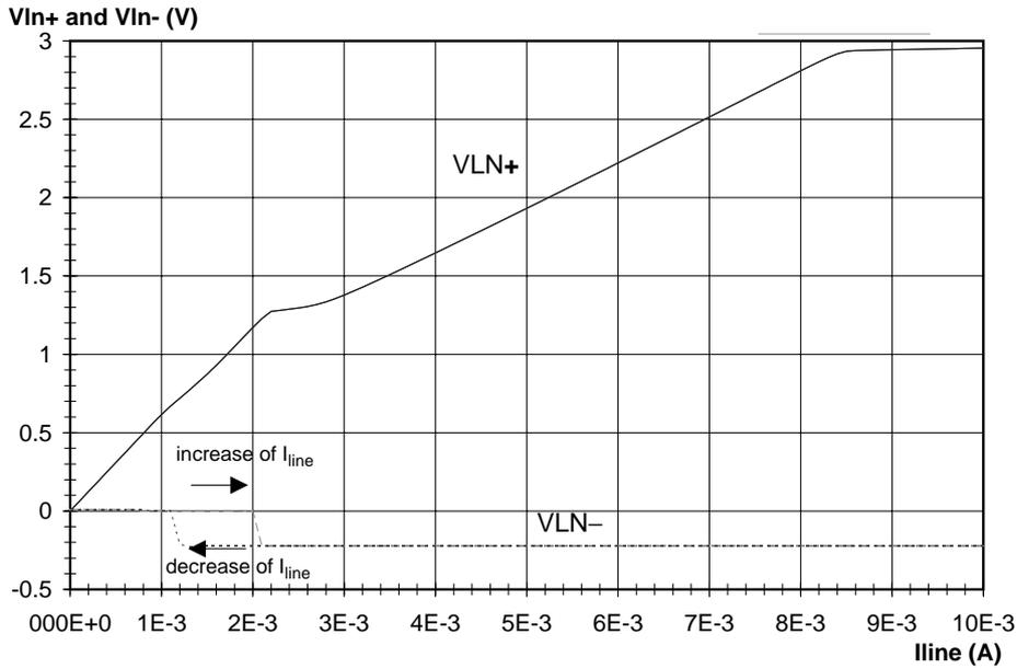
Fig.8 The voltage on VLN+ and VLN- both wrt GND versus  $I_{line}$  at VRM at low  $I_{line}$
