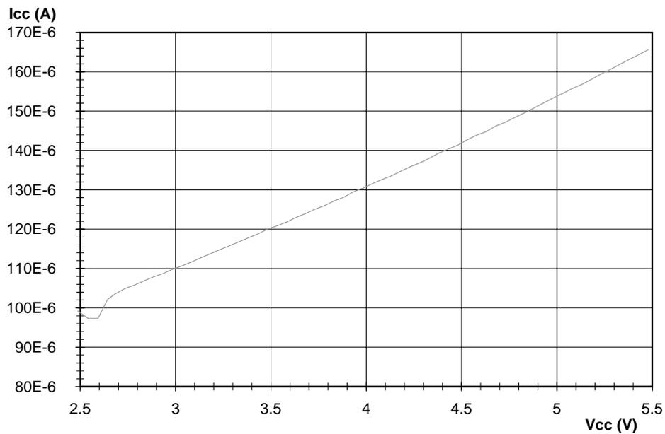
Fig.41 Current consumption I<sub>CC</sub> versus V<sub>CC</sub> at power down; PD = 1
