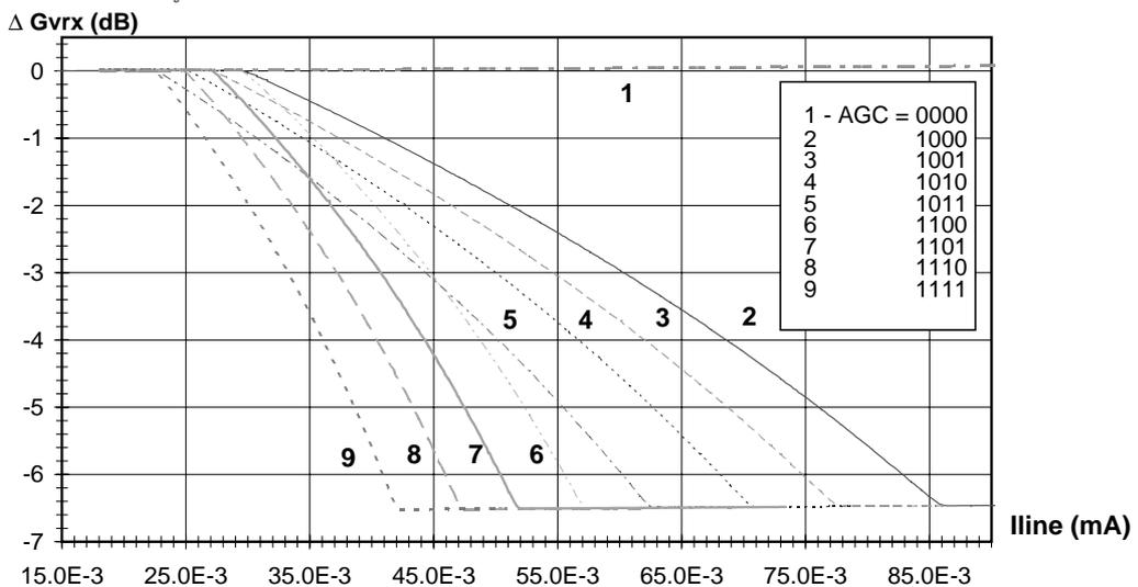
Fig.26 AGC control of the RX amplifier
