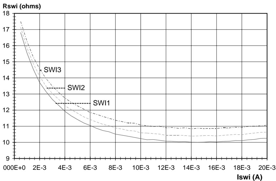
Fig.38 Dynamic resistance of the SWI-switches versus current
