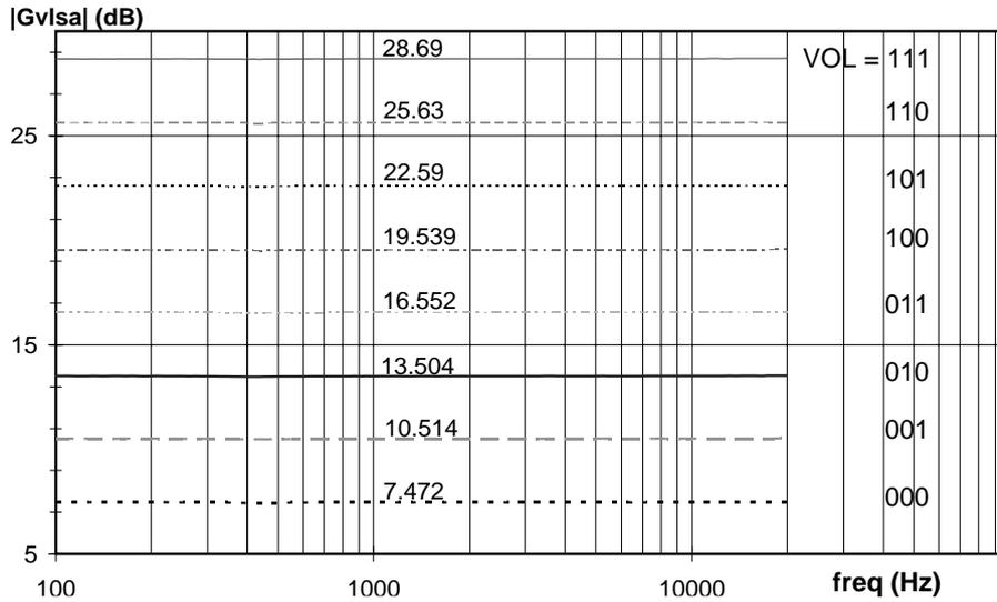
Fig.37 LSA gain versus VOL control setting
